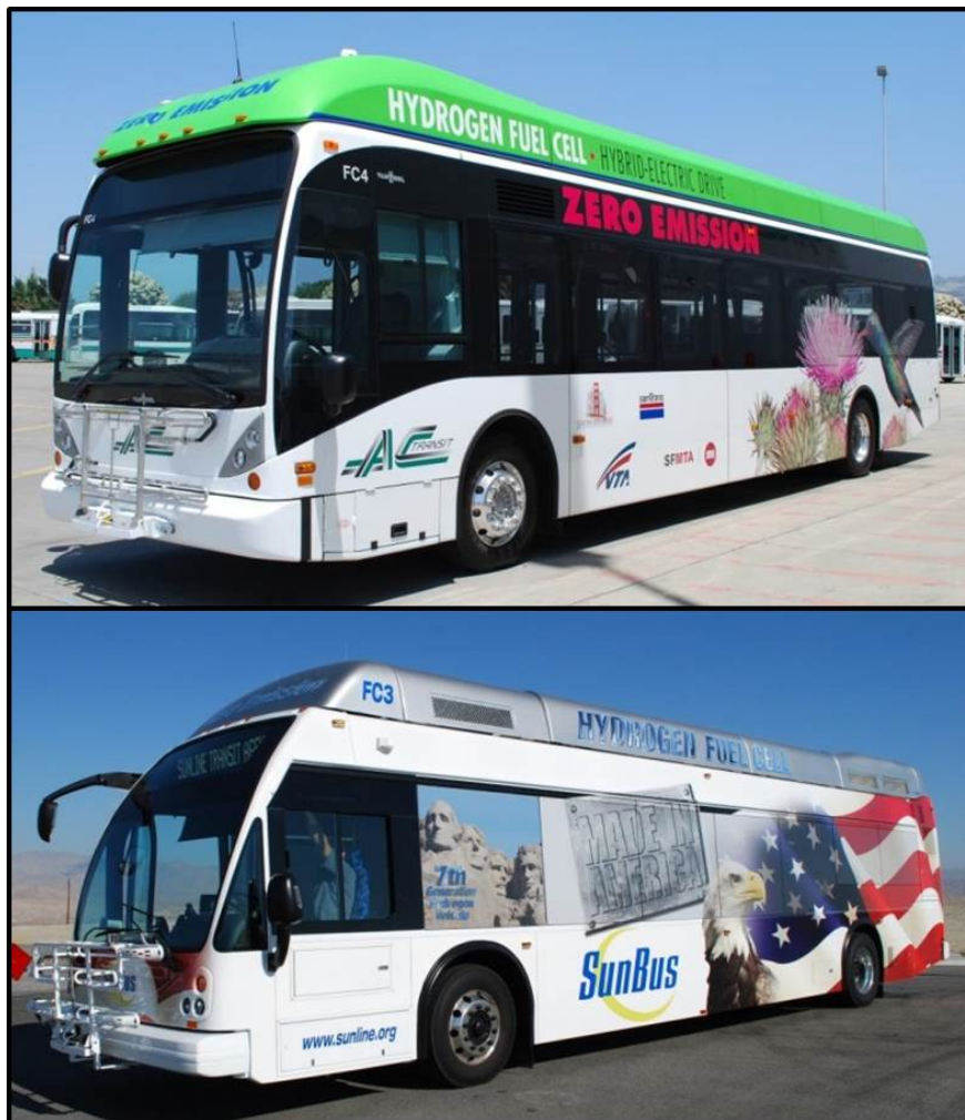
Figure 2. FCEBs at TRL 7: AC Transit ZEB FCEB (top) and SunLine AFCB (bottom)
