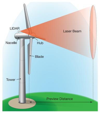
Using laser technology known as a light detection and ranging system, or lidar, NWTC researchers can provide a look-ahead capability. The lidar allows the turbine to effectively "brace itself" for a wind gust before that gust actually arrives, measuring wind speed approximately 50 to 100 meters ahead of the turbine. *Illustration by Al Hicks, NREL*
