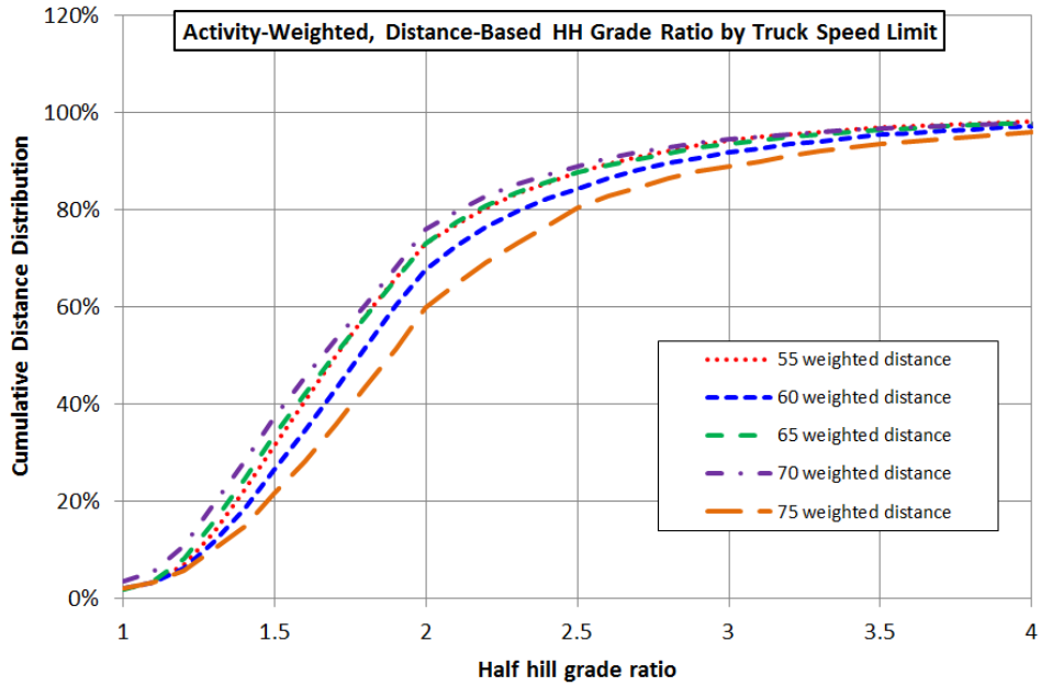
Figure B8. Activity-weighted distance-based cumulative distributions of half hill grade ratio (maximum to average half hill grade) by truck speed limit
