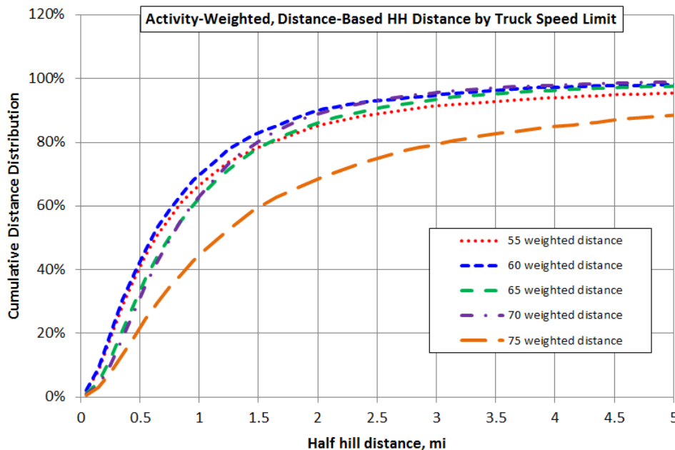
Figure 26. Activity-weighted, distance-based cumulative distributions of half hill distance by truck speed limit
