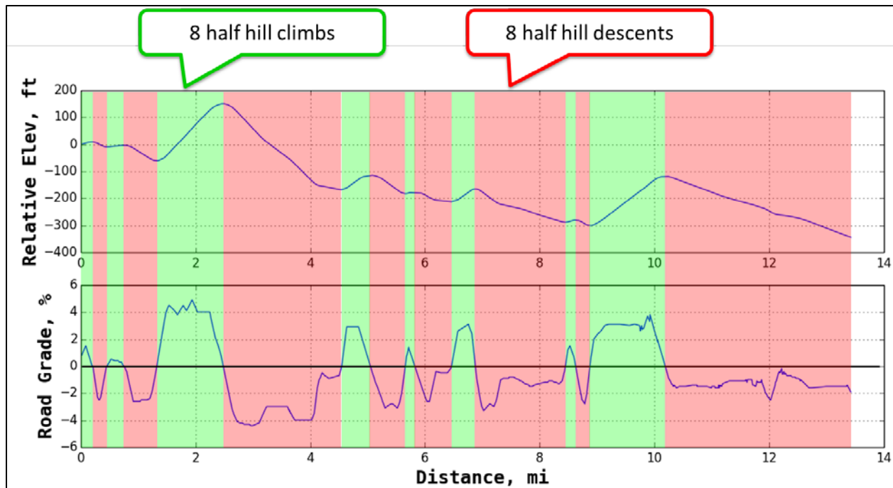
Figure 18. Example section of controlled access highway broken into 16 half hills (eight climbs and eight descents)
