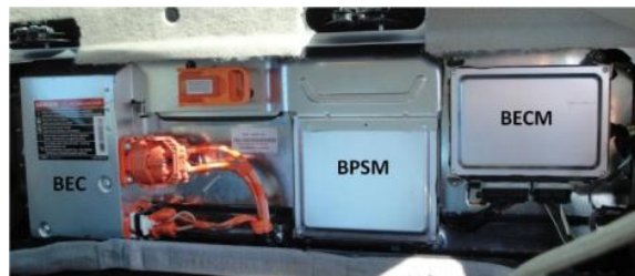
Figure 1. Photo of Fusion Hybrid HVTB. Image by John Ireland, NREL
