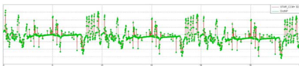
Figure 7. Comparison of lumped electrochemistry model vs three dimensional electrochemistry model over a 30min drive cycle (Voltage scale removed)
