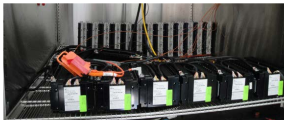
Figure 3. JSR LIC modules in environmental chamber during bench testing, with production 2012 Fusion Hybrid NiMH modules in the background. Image by John Ireland, NREL
