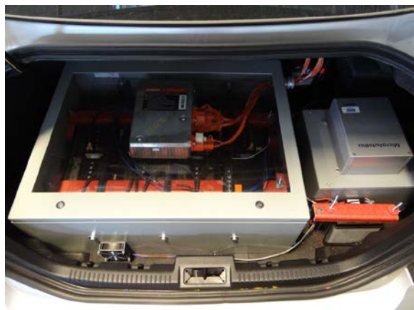
Figure 4. Fully-integrated conversion system mounted in the trunk of the Fusion Hybrid test platform. Image by Jon Cosgrove, NREL
