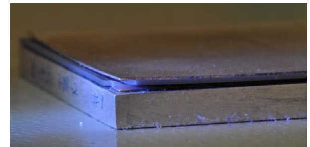
Substrate Delamination and Cracking
