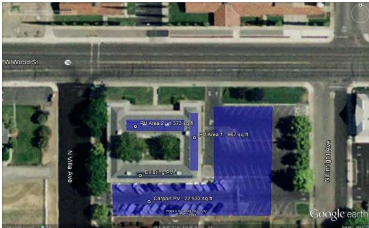
Figure 6-5. Proposed PV system locations at Reclamation’s Willows building (highlighted in blue) Willow’s staff indicate the carport is not feasible at this time due to operational space requirements. Source: Google Earth (modified by Otto VanGeet, NREL)
