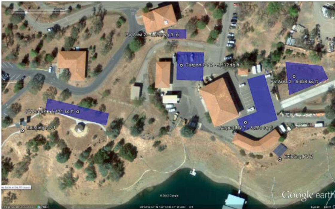
Figure 6-13. Proposed PV system locations at Reclamation’s Lake Berryessa site (highlighted in blue)
