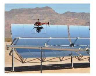
A high-performance radio-controlled helicopter, holding a specialized camera, is part of the Distant Observer photogrammetric data acquisition system. Here, the helicopter hovers over a trough in the Nevada Solar One CSP plant outside of Las Vegas. Photo by NREL Distant Observer Team, NREL/PIX 23115 Highlights in Research & Development
