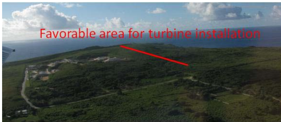
Figure 13. Slight ridge to the east of the quarry on southern Saipan that could allow the installation of a single line of wind turbines
