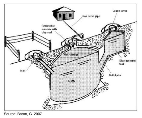
Figure 10. Fixed dome biogas plant design
