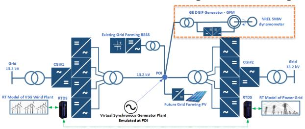
Main Objective: Development, implementation and validation of GFM controls using GE generator/converter platform with NREL's 5 MW dynamometer and Controllable Grid Interfaces
