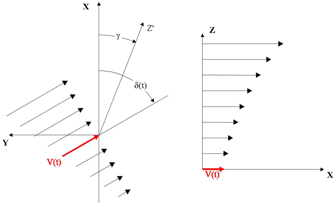
Figure 7.1 Wind shear and direction models: Overhead view of horizontal shear in left sketch; Cross-section view of vertical shear in right sketch. Note the wind direction ( $\delta$ ) and yaw angle ( $\gamma$ ) are both defined with respect to the **X** axis (global direction indicating zero yaw and wind direction angles). All directions and shears are shown in their positive sense.
