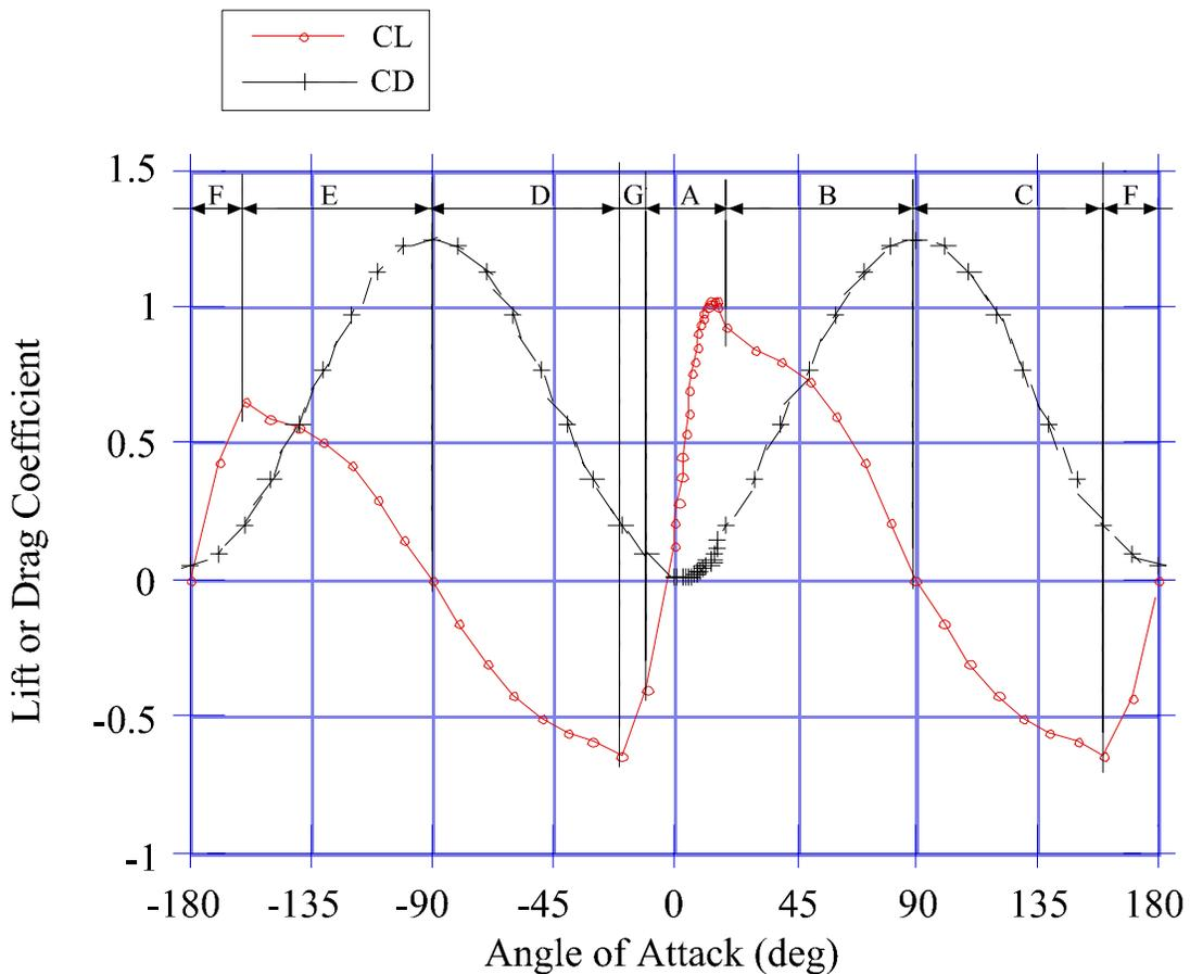
Figure D1. Lift and drag coefficients for a typical airfoil.
