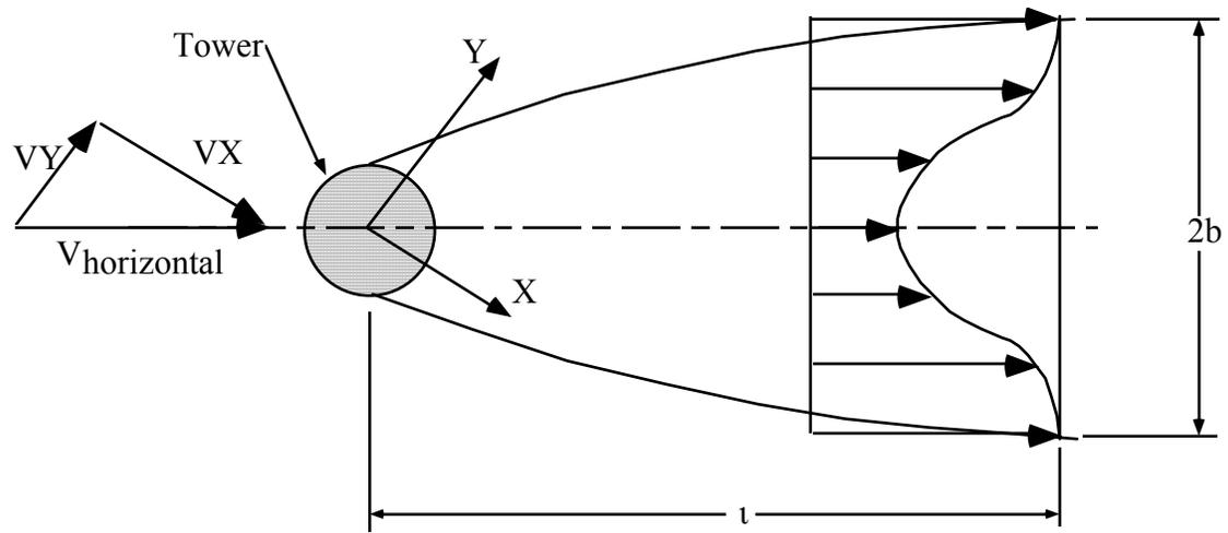
Figure A1. Schematic of the tower shadow model with a cross flow ( $V_Y$ ). The tower wake decays in strength and grows in width as the distance from the tower,  $t$ , increases. The strength and half-width are specified at a reference position, a distance  $L_S$  from the tower center.
