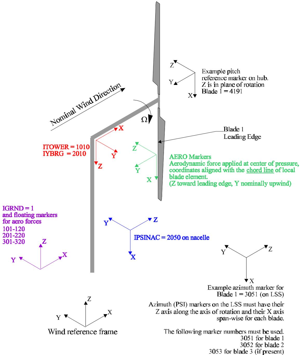
Figure 4.1 Required marker identification and orientation
