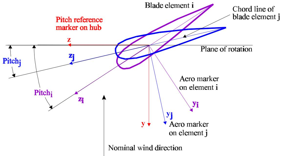
Figure 4.2 Definitions of aerodynamic pitch. The pitch angle determined by ADAMS for each blade element. The angles are shown in their positive sense. The  $y$  and  $z$  coordinates show the GFORCE marker orientations for two different blade elements  $i$  and  $j$
