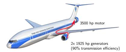
Turboelectric propulsion system has an electric BLI propulsor powered by generators mounted on the under-wing turbofans
