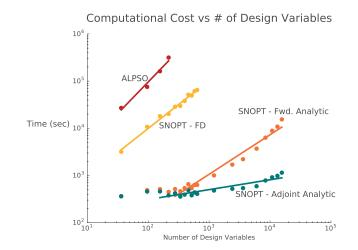
We want to design complex systems with coupled multi-fidelity models, so we use gradient based optimization with analytic derivatives
