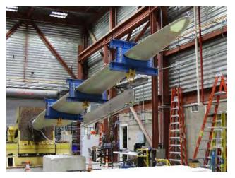
13-m TP Blade static load testing at 100% design load (PhotoCredit: NREL)
