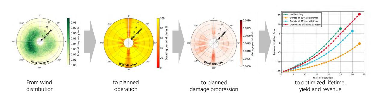
→Only the combination of multiple models allows for computation of trade-off between energy and damage
