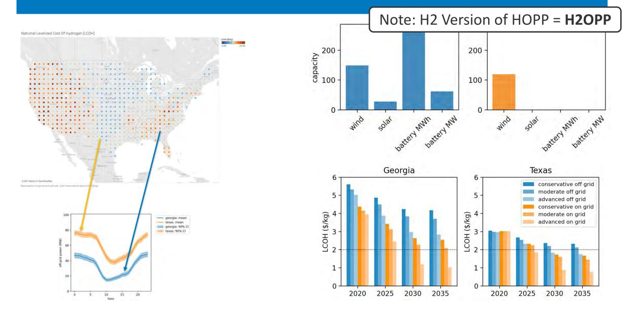
Each result is using the optimal plant + electrolyzer size for that location (resource) and cost scenario
