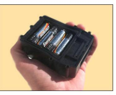
participants to turn the unit on or off. The devices were placed in the windshield, or other area where signal would not be disrupted. If the vehicle had a working cigarette lighter, ETC Institute connected the GPS device to the lighter to provide backup power in the event the batteries failed.
