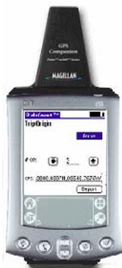
Figure 3-1: GPS-Enhanced Palm Device for On-Board Counts
