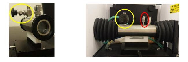
Figure 3. IR gas cell used for kinetic measurements from two different angles. The path length through the cell is 11 cm, and the KBr windows are 25 mm in diameter by 2 mm thick from Sigma Aldrich. The injection port (circled in red) is sealed with a septum, and the outgas port (yellow) can be opened for purging, if necessary.
