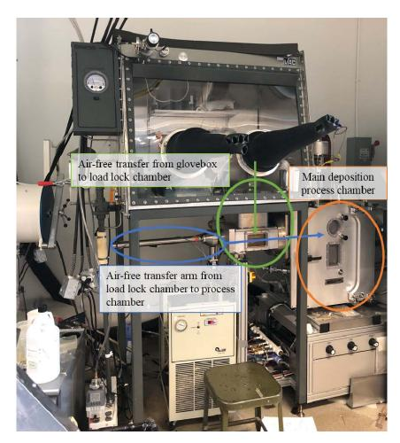
Figure 4. Sputter system and sample transfer process.
