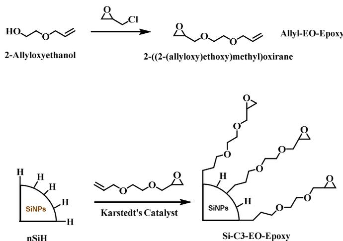
**Figure 22.** Synthesis of functional precursor containing an epoxy group and its hydrosilylation reaction with silicon-H terminated Si NPs.
