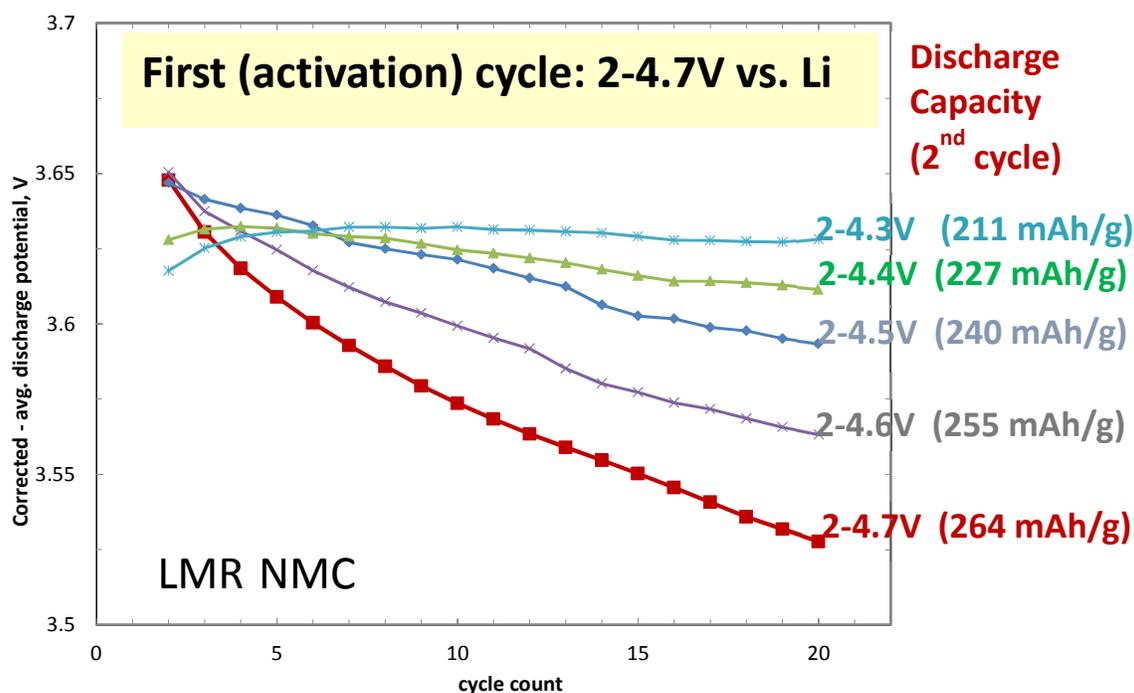
Figure 20. Capacity of LMR-NMC Cathodes as a function of upper cutoff voltage of  $\text{Li}_{1.2}\text{Ni}_{0.25}\text{Mn}_{0.55}\text{Co}_{0.10}\text{O}_2$  while using a graphite anode.
