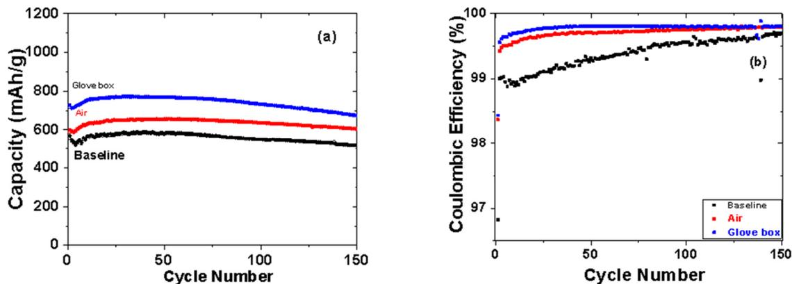
Capacity retention (lithiation: solid; delithiation: empty) and (b) the Coulombic efficiency of silicon-graphite/Li cells.
