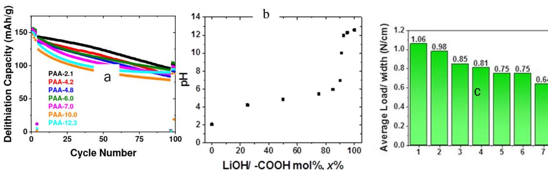
Figure 8. (a) Specific delithiation capacity profiles for NCM523/silicon-Gr full cells containing lithiated PAA binders with different pH values. (b) Equivalence curve for the lithiation of the PAA Binder. (c) Average load/width with a range of 50 mm for silicon-Gr electrodes. Numbers correspond to the pH samples (1= lowest (pH= 2.1), 7 = highest (pH = 12.3)).
