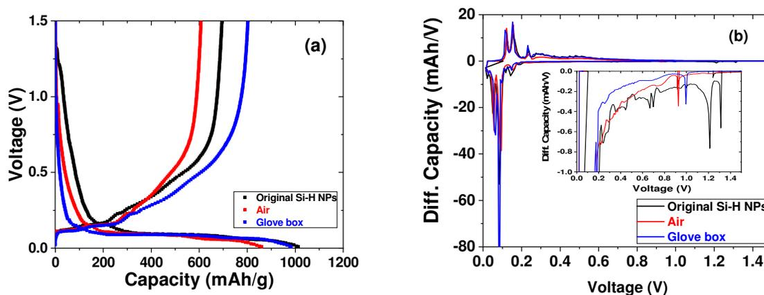
**Figure 24.** (a) The 1<sup>st</sup> formation cycle voltage profiles and (b) differential capacity profiles (dQ/dV) of electrodes based on pristine Si NPs, Si NPs synthesized in air and in glovebox (inset is an expansion of the dQ/dV plot during the lithiation process).
