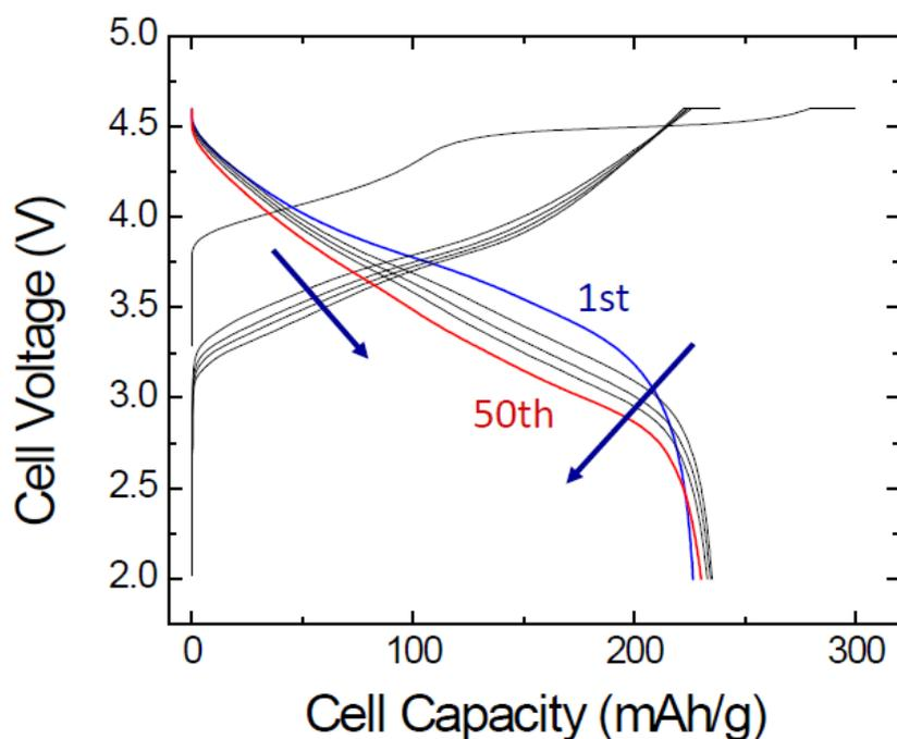
Figure 19. Capacity fade of the cathode sample associated with gradual defect consolidation and cation movement in the lattice.
