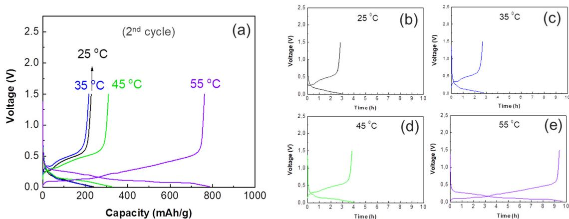
Figure 5. (a) Voltage versus capacity for the second cycle (after the three first formation cycles) of silicon/Gr half-cells and their corresponding voltage versus time plots at (b) 25, (c) 35, (d) 45 and (e) 55 °C. In all the cases the silicon-graphite electrode was from CAMP (A-A013).
