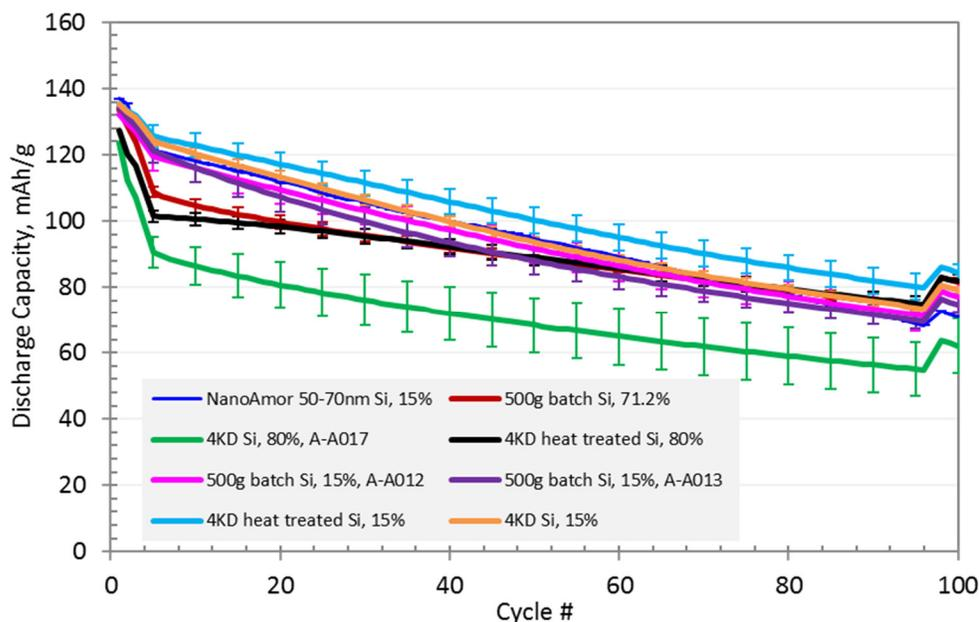
Figure 18. Full cell results using the silicon deep dive protocol for the high-silicon graphite-free anodes and 15 wt.% Si in graphite composite. All anodes were tested against a capacity-matched NMC532 cathode. The anode to cathode capacity pairing for the electrode couples was based on
