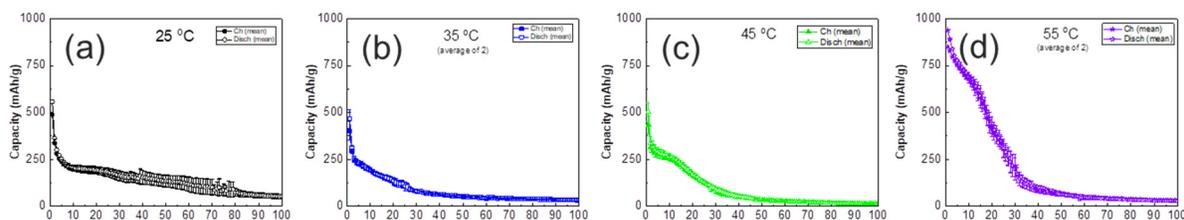
Figure 4. Charge and discharge capacity *versus* cycle number plot of silicon/Gr half-cells containing Gen 2 electrolyte and cycled at (a) 25, (b) 35, (c) 45 and (d) 55 °C. The filled and empty markers represent, respectively, the charge and discharge capacities. In all the cases the silicon/Gr electrode was from CAMP (A-A013).
