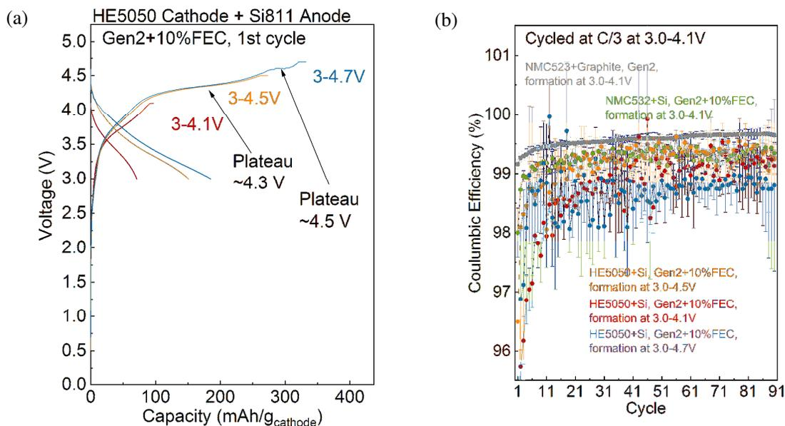
Figure 21. (a) Electrochemical evaluation of a silicon-rich electrode (silicon811) versus upper cutoff voltage for a HE5050 cathode. (b) Coulombic efficiencies of a silicon-rich electrode versus HE5050 using the window a 4.1 Upper Cutoff Voltage, but various windows (up to 4.7V) for formation cycling.
