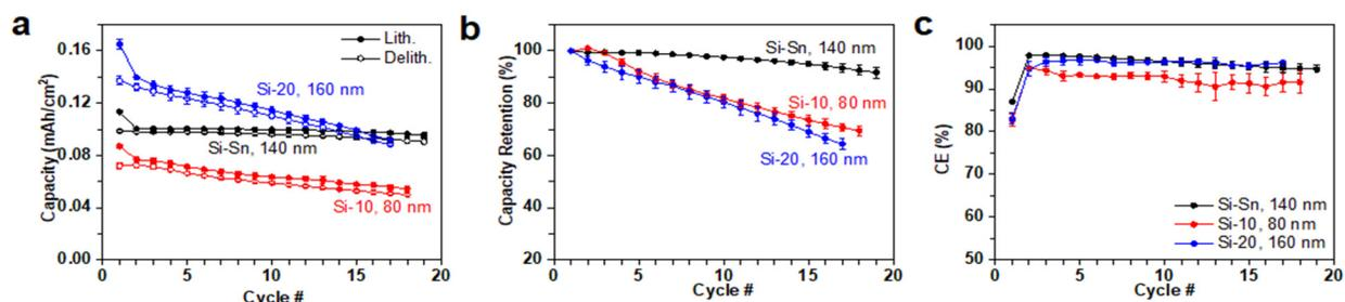
Figure 13 (a) Capacity, (b) capacity retention and (c) CE of Si-Sn and Si films of similar thickness.
