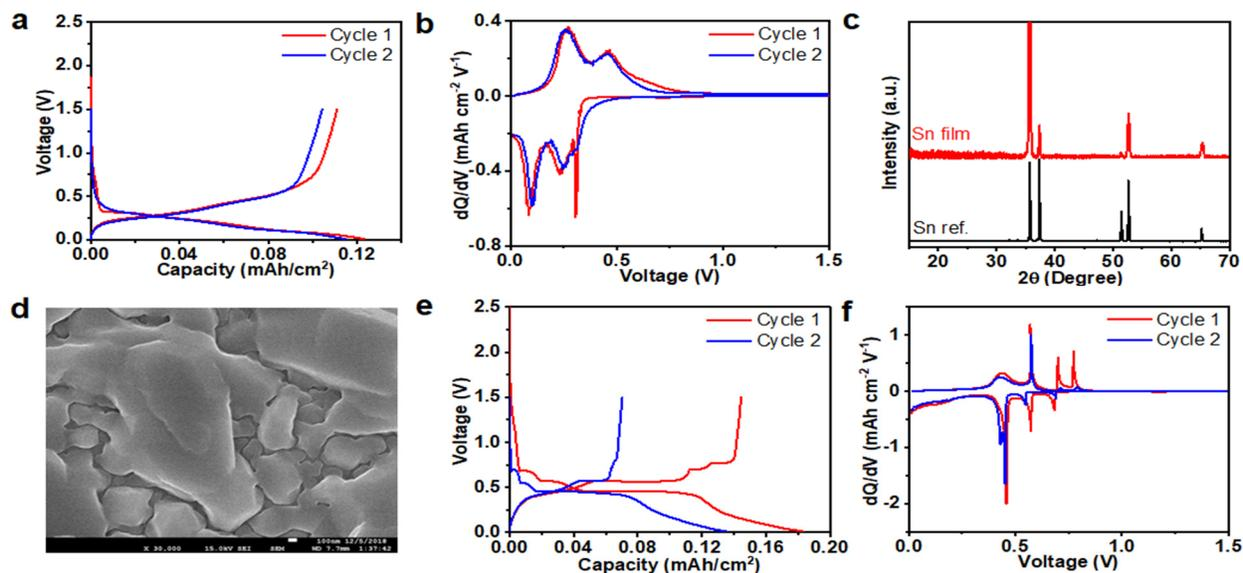
Figure 12 (a) Voltage profiles and (b) dQ/dV plots of Si film, (c) XRD, (d) SEM image, scale bar is 100 nm, (e) voltage profiles and (f) dQ/dV plots of Sn film.
