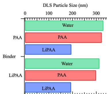
Figure 11. Particle sizes of silicon-Gr-CB anode slurries measured using Dynamic Light Scattering (DLS)
