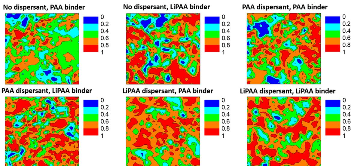
Figure 7. Raman maps of the relative fraction of silicon across electrodes processed using different dispersants and binders. Each map is 50  $\mu\text{m}$  x 50  $\mu\text{m}$  and represents 2500 spectra collected at 1  $\mu\text{m}^2$  resolution. The most uniform distribution of silicon is obtained when LiPAA is used as a dispersant.
