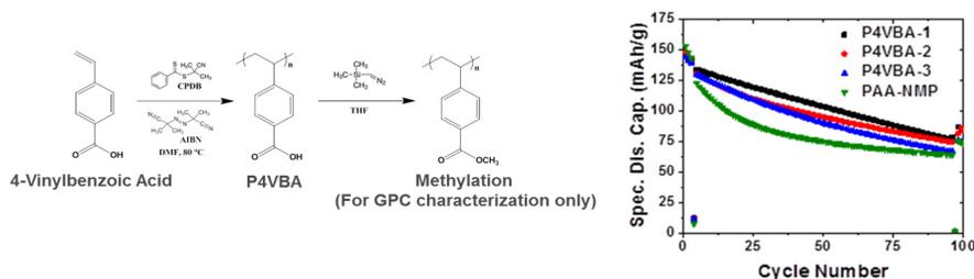
Figure 9. Synthesis route for the P4VBA-based binders and their cycling stability with an NMC 532 cathode
