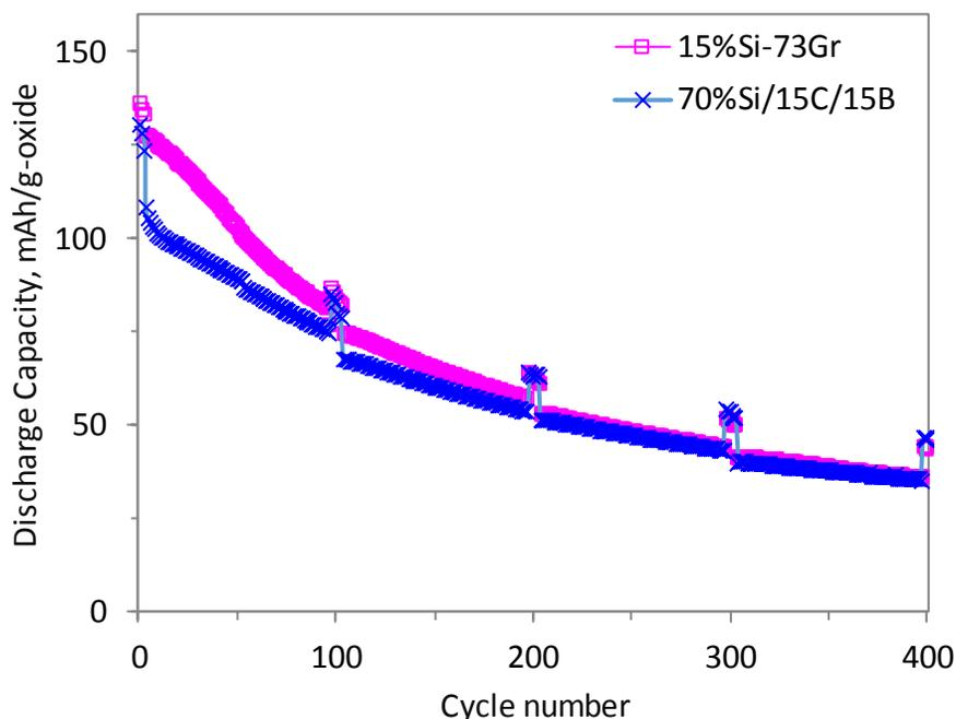
Figure 15. Discharge capacity vs. cycle number for an NCM523/15Si cell (magenta plot) and an NCM523/70Si cell (blue plot) tested at 30°C. The test protocol contained four repetitions of 100 cycles. In each of these 100 cycles, cycles 1-3 are at a ~C/20 rate, 4-97 are at a ~C/3 rate and 98-100 are at a C/20 rate.
