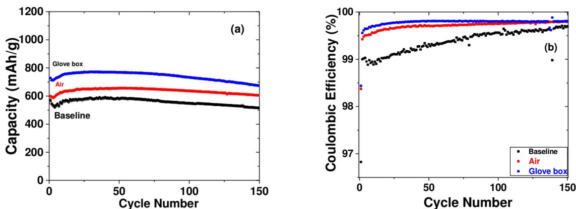
**Figure 25.** (a) Capacity retention (lithiation: solid; delithiation: empty) and (b) the Coulombic efficiency of silicon-graphite/Li cells.
