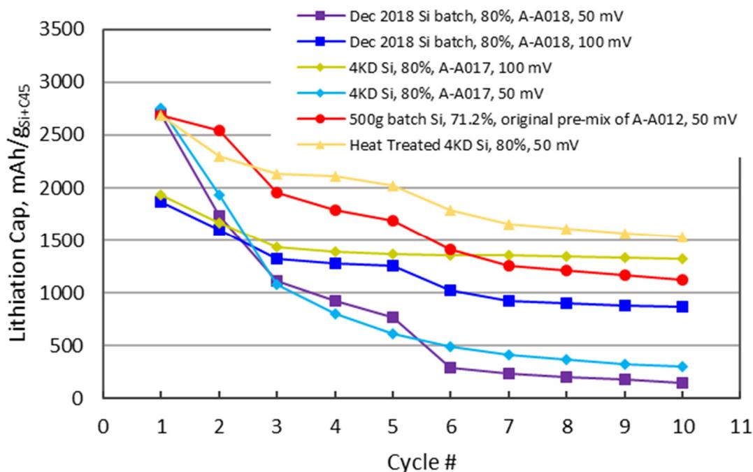
Figure 17. Lithiation capacity versus lithium metal for various graphite-free silicon electrodes fabricated by the CAMP Facility. These cells were cycled between 0.05 to 1.5 V or 0.1 to 1.5 V vs. Li<sup>+</sup>/Li as noted in the legend.
