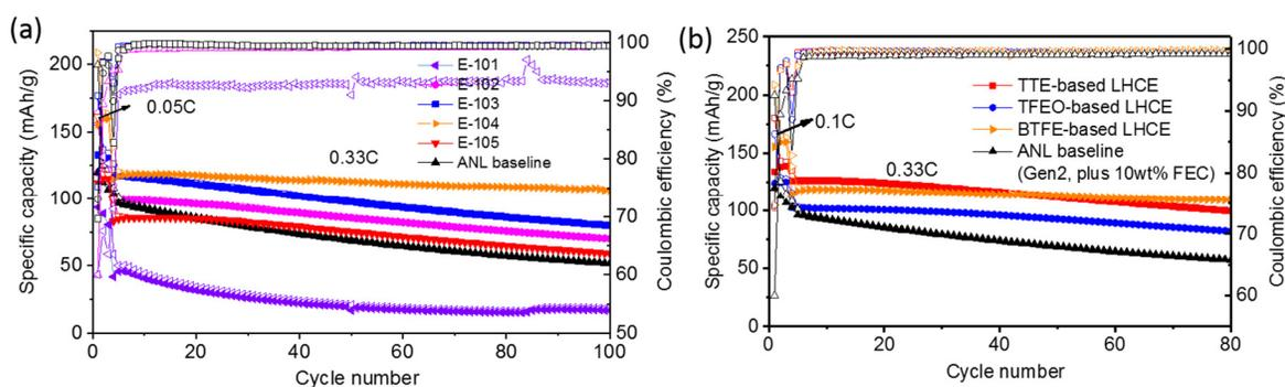
Figure 6. a) Cycling performance of NMC532 || silicon/Gr (CAMP electrodes) in BTFE-based electrolytes with different salt concentration; b) cycling performance of NMC532 || silicon/Gr (CAMP electrodes) in BTFE, TTE and BTFE-based electrolytes.
