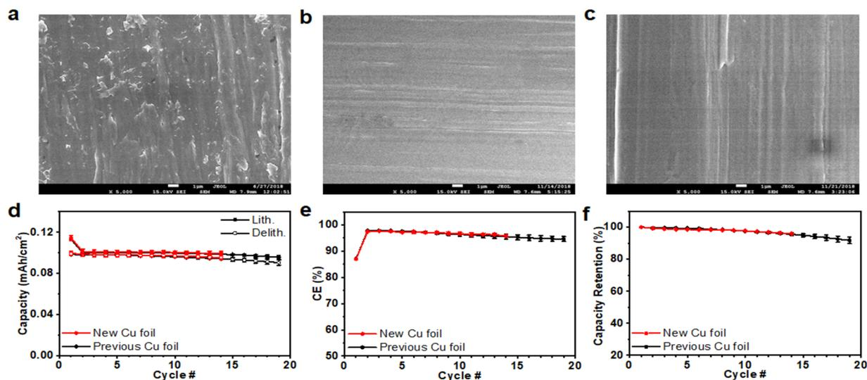
Figure 1 SEM images of (a) previous Cu foil, (b) new Cu foil and (c) Si-Sn film on new Cu foil, scale bar is 1  $\mu$ m. Comparison of Si-Sn films on previous and new Cu foil: (d) lithiation/delithiation areal capacity, (e) CE and (f) capacity retention upon cycling.
