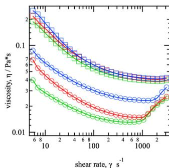
Figure 10. Rheological characterization of silicon-Gr-CB anode slurries: LiPAA dispersant– Blue, PAA dispersant – Red, No dispersant – Green. Circles – PAA binder, Squares – LiPAA binder added.
