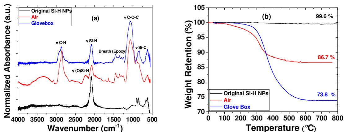
**Figure 23.** (a) FTIR spectra and (b) TGA thermograms of the epoxy-functionalized Si NPs. (*Black*: pristine Si NPs, *Red*: Si NPs synthesized in air, and *Blue*: Si NPs synthesized in Ar-filled glovebox).
