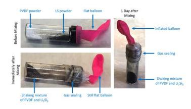
Figure 2. Images of gas-cathcing setup before, immediately after, and 1 day after the mixing of PVDF and Li<sub>7</sub>Si<sub>3</sub>.
