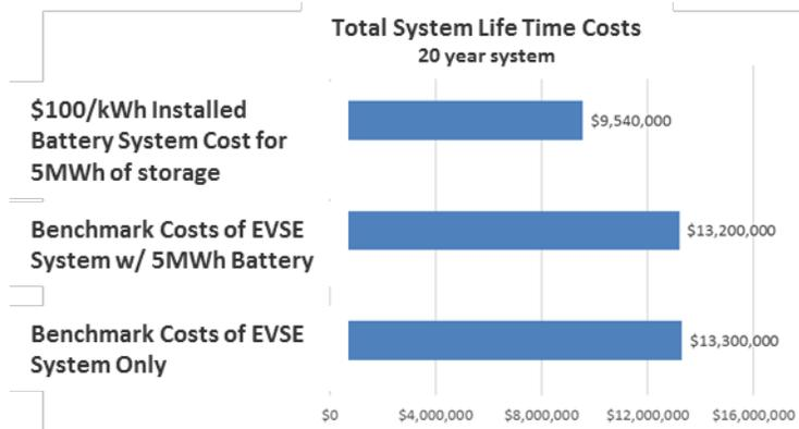
Figure 7. Total lifetime time cost estimates based upon 20 year life, relative to demand current demand charges and current battery cost vs \$100KWh targets.
