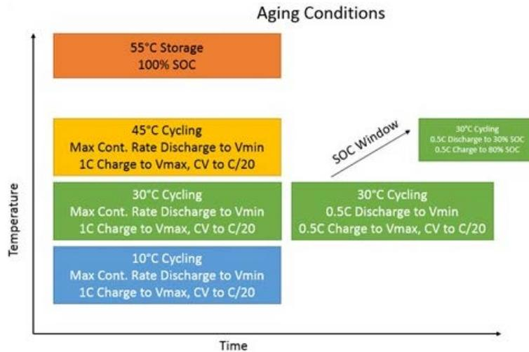
Figure 8. Test matrix for cells under baseline scenario.
