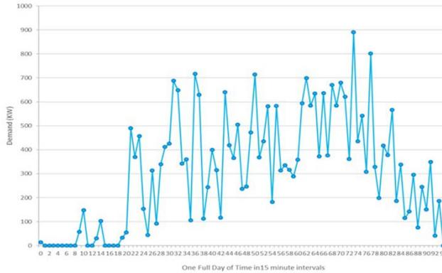
Figure 5. Six EVSE (350 kW each) power-station demand profile.
