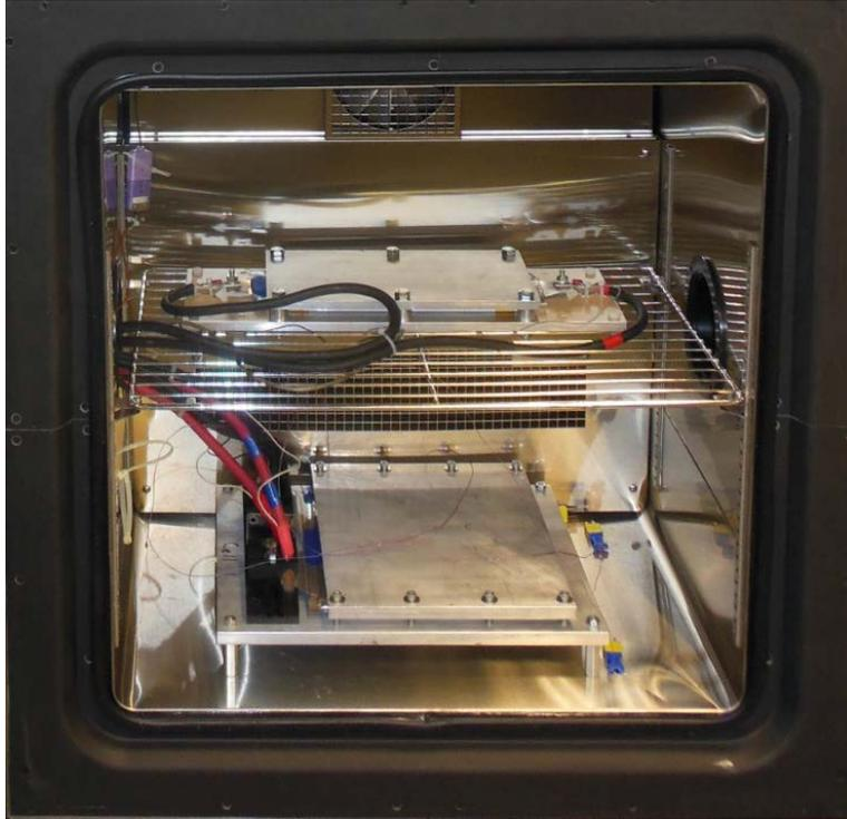
Figure 9. LG Chem cell (top) and XALT cell (bottom) sharing 45 °C test chamber.
