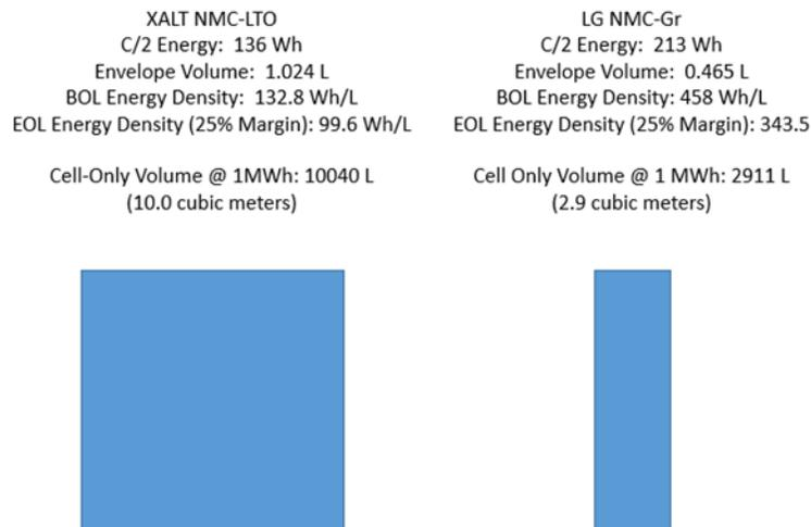
Figure 10. Comparison of energy density of two cell technologies being tested.
