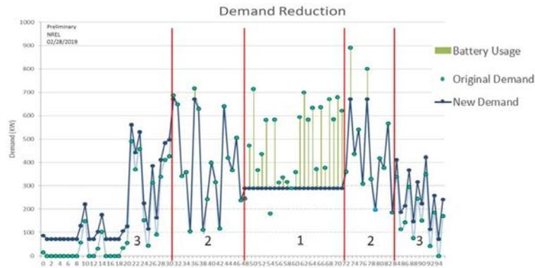
Figure 6. Demand change with the use of battery storage.
