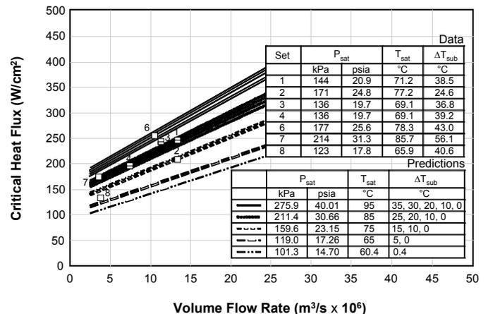
Fig. 9 Comparison of CHF predictions and experimental data.
