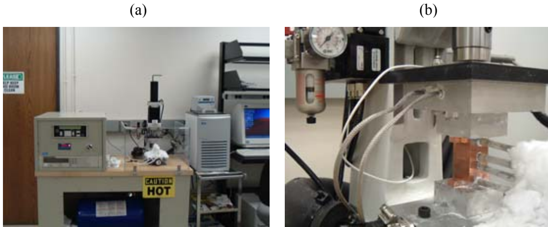
Figure 2. Test apparatus for thermal resistance measurements: (a) facility setup at NREL, (b) apparatus
