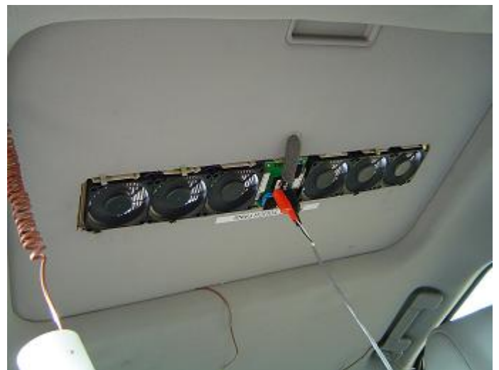
Figure 1. Test (Non-Production) Installation of the Solar-Powered Parked Car Ventilation System
