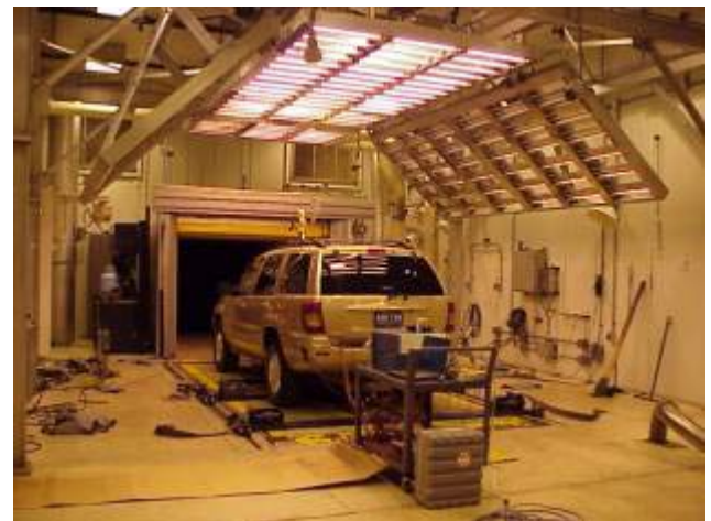
Figure 4. Test Cell with IR Lamps
