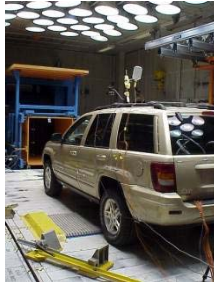
Figure 3. Test Cell with Metal Halide Lamps
