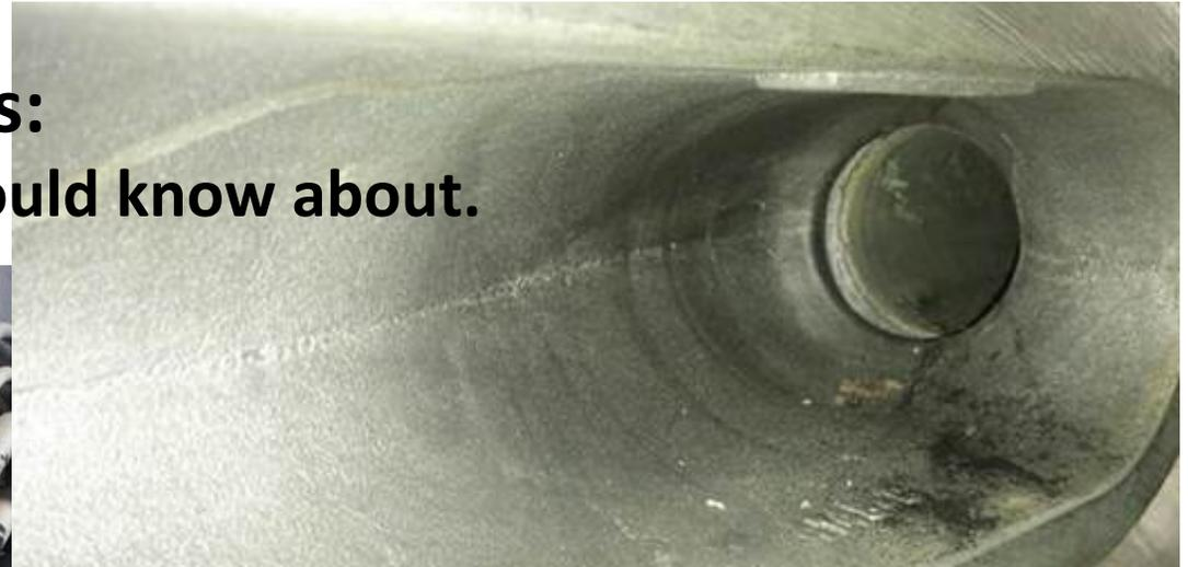
**Inside:** Insulation shavings left from abrasion caused by thermal expansion and contraction of conduit. Use of protective plastic cuff unknown.
