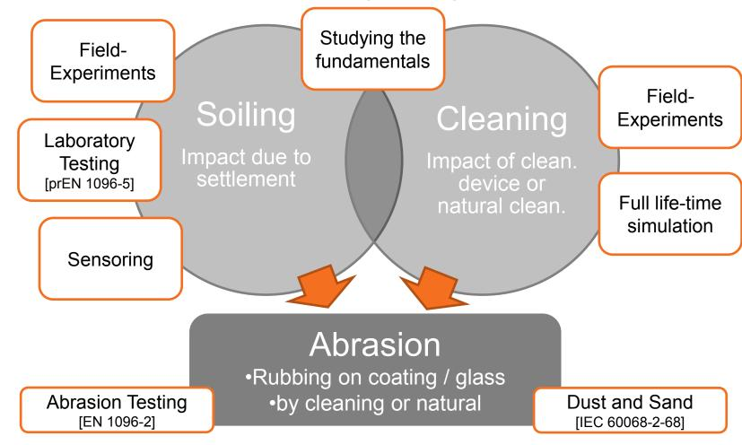
→ Aim: Simulation of realistic soiling, cleaning and abrasion conditions
