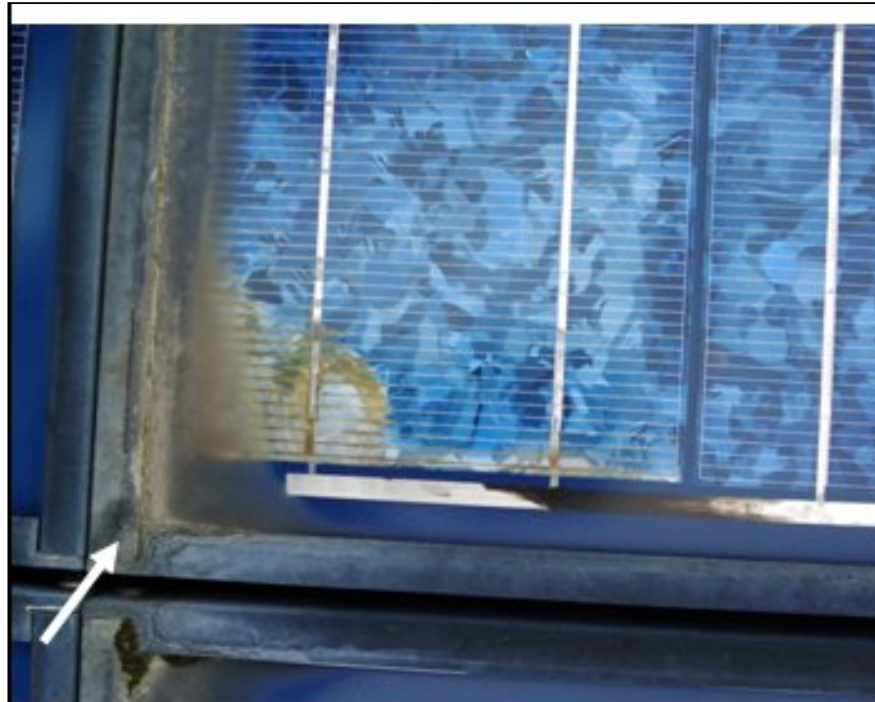
A 20y-field-aged PV module with delamination failure and induced corrosion
