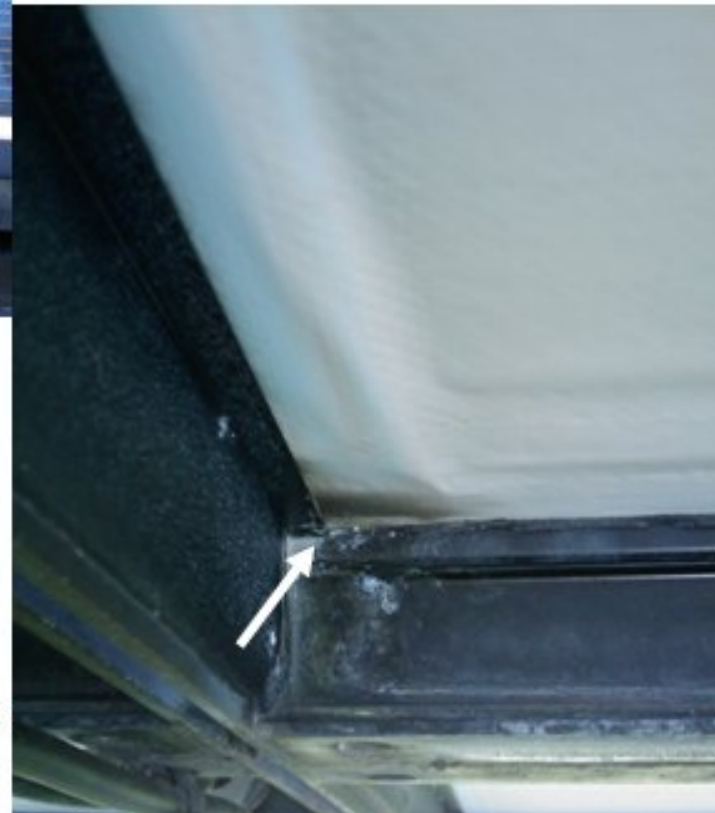
A 20y-field-aged PV module with delamination failure and induced corrosion
