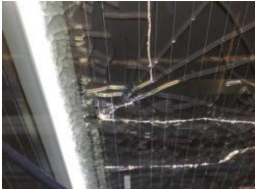
Module back glass cracked due to rock from mowing equipment.
