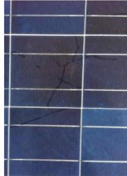
**Snail trails and microcracks observed on installed modules.**
