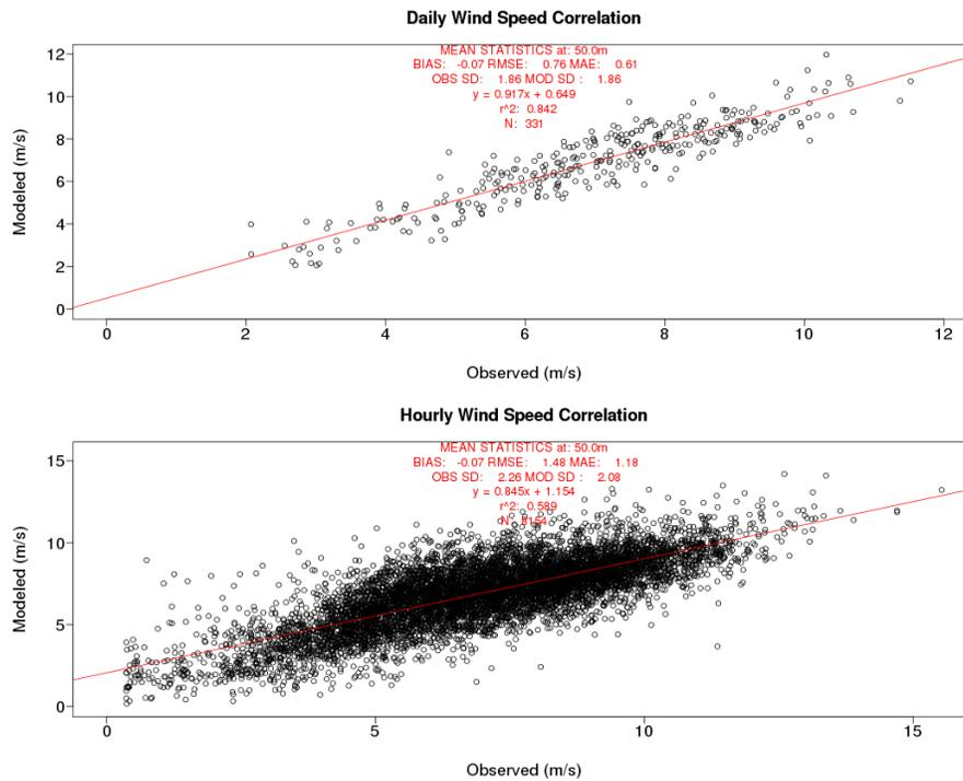
**Figure 2a.** Scatter plots of observed and WRF-generated daily average (top) and hourly average (bottom) wind speeds at the Longford tower for 2013.
