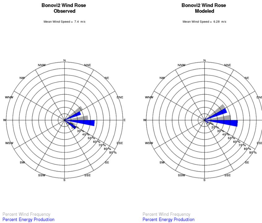
**Figure 1b.** Observed (left) and WRF (right) wind roses for the Bovoni2 tower, for 2013.
