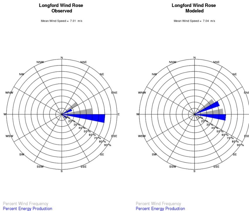
**Figure 2b.** Observed (left) and WRF (right) wind roses for the Longford tower for 2013.
