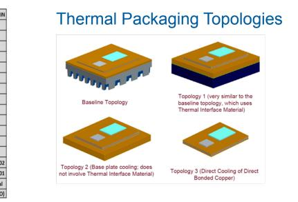
Developed basic framework for rapid assessment of interactions between thermal packaging topologies, materials, and thermal performance.
