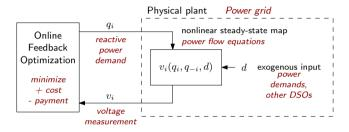
Interconnection of optimization iteration (e.g., projected gradient flow) with the real plant
