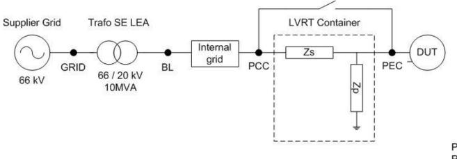
PCE. Point of especimen coupling PCC. Point of common coupling BL. 20kV Bus LEA Zs. Serial impedance Zp. Parallel impedance DUT. Device under test
