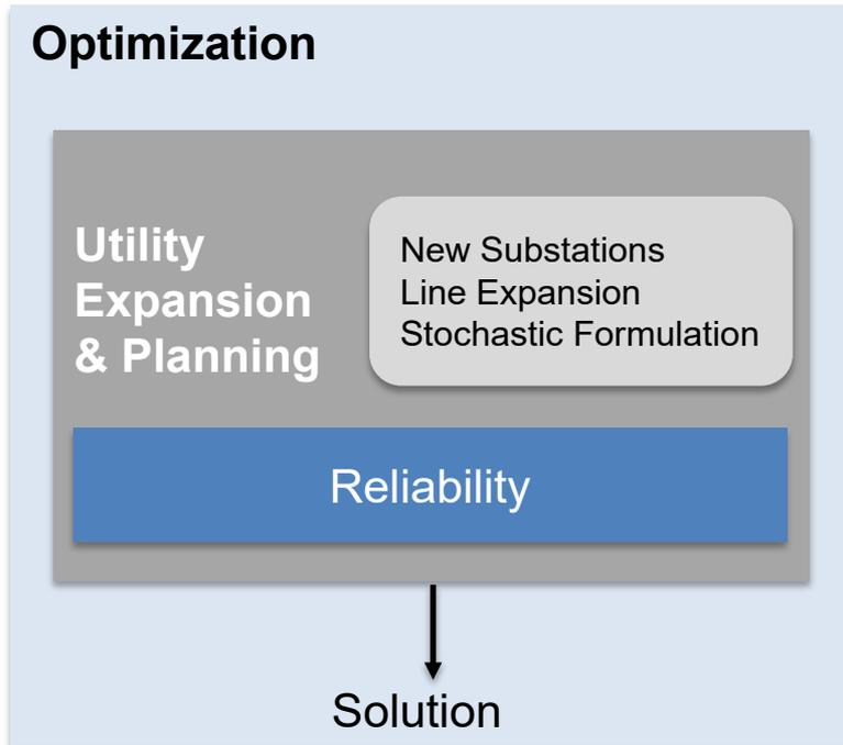
**Reliability** is explicitly included in the expansion and planning optimization model by considering the expected value of loss of load in the different nodes of the network.
