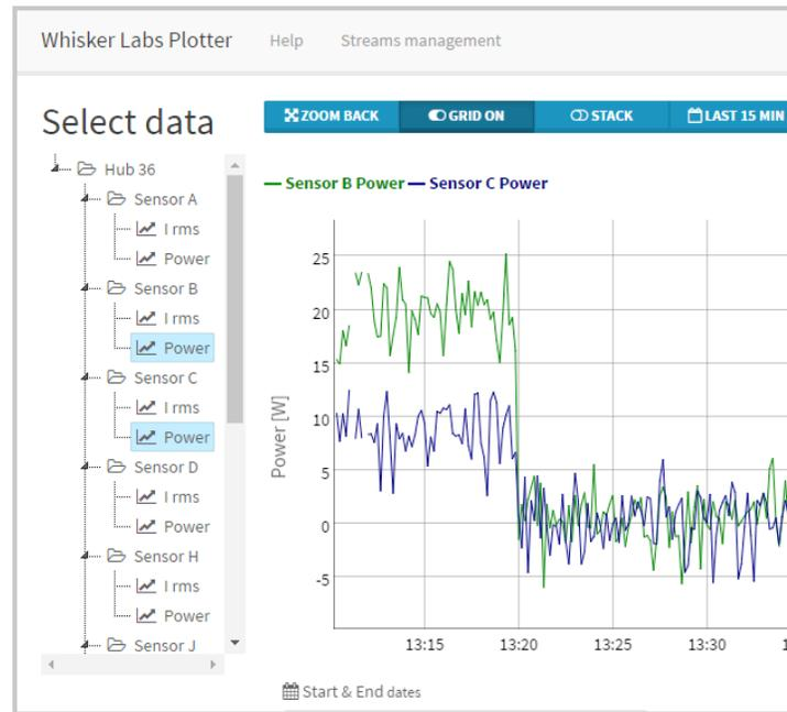
Whisker Labs' plotting interface shows circuit-level power, voltage, and current information via the Web.
