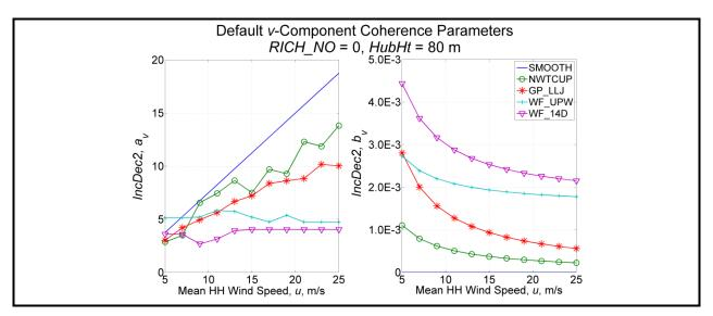
Figure 14. Default *v*-component coherence parameters, *IncDec2*, ( $a_v$  left,  $b_v$  right) as a function of wind speed, using *RICH\_NO* = 0 and *HubHt* = 80 m (IEC does not define *v*-component coherence parameters)
