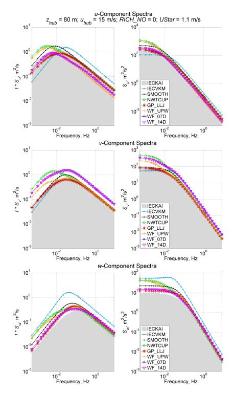
Figure G-2. Neutral velocity spectra for the 8 spectral models available in TurbSim, using a 15 m/s wind speed at 80 m; IECKAI and IECVKM use NTM category "B" and 61400-1 3<sup>rd</sup> ed. scaling; the non-IEC models use *RICH\_NO* = 0 and *UStar* = 1.1 m/s
