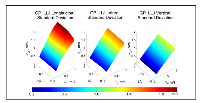
Figure 20. GPLLJ-model stable/neutral turbulence as a function of local stability and shear velocities
