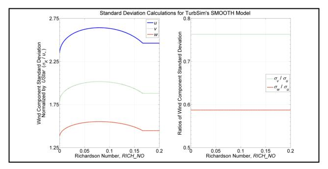
Figure 18. SMOOTH-model stable/neutral turbulence as a function of *RICH\_NO*: left: standard deviation normalized by *UStar.* right: Relationships between components' standard deviations
