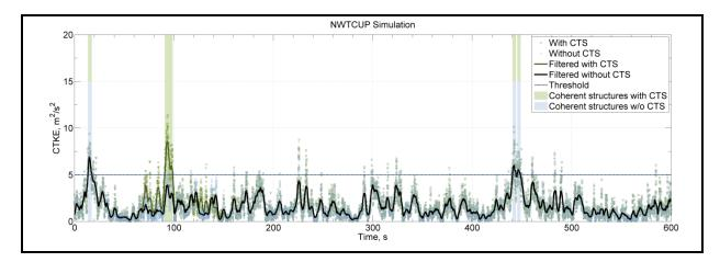
Figure 26. Example time series from the NWTCUP model: the black line indicates the background wind file; the green shows the addition of events in a coherent time-step file (".cts")
