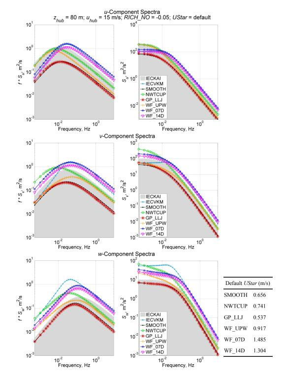
Figure G-5. Unstable velocity spectra using a 15 m/s wind speed at 80 m; the non-IEC models use *RICH\_NO* = -0.05 and *UStar* = "default"; the IEC models, which are neutral (*RICH\_NO* = 0), were added for reference; they use NTM category "B" and 61400-1 3<sup>rd</sup> ed. scaling
