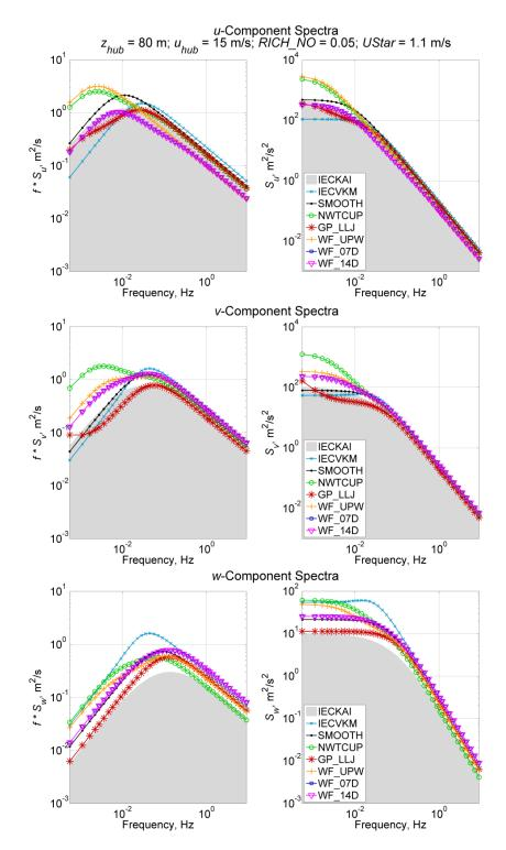
Figure G-4. Stable velocity spectra using a 15 m/s wind speed at 80 m; the non-IEC models use RICH\_NO = 0.05 and UStar = 1.1 m/s; the IEC models, which are neutral (RICH\_NO = 0), were added for reference; they use NTM category "B" and 61400-1 3<sup>rd</sup> ed. scaling
