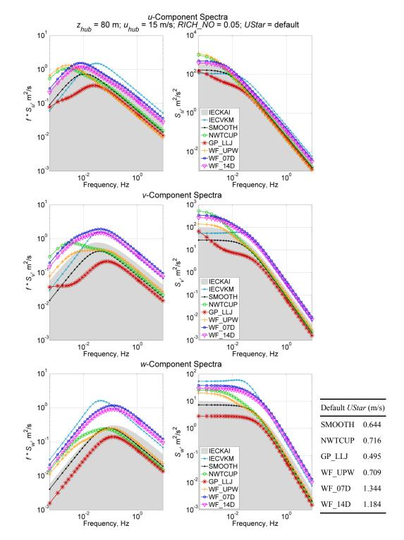
Figure G-3. Stable velocity spectra using a 15 m/s wind speed at 80 m; the non-IEC models use *RICH\_NO* = 0.05 and *UStar* = "default"; The IEC models, which are neutral (*RICH\_NO* = 0), were added for reference; they use NTM category "B" and 61400-1 3<sup>rd</sup> ed. scaling
