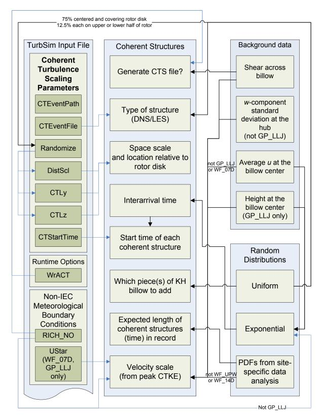
Figure C-8. Parameters for coherent structures and the Coherent Turbulence Scaling Parameters section of the TurbSim input file; the SMOOTH model uses the GP\_LLJ scaling
