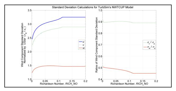
Figure 19. NWTCUP-model stable/neutral turbulence as a function of *RICH\_NO*: left: standard deviation normalized by *UStar*, right: relationships between components' standard deviations
