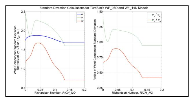
Figure 22. WF\_07D- and WF\_14D-model stable/neutral turbulence as a function of *RICH\_NO*: left: standard deviation normalized by *UStar*, right: ratios of standard deviations
