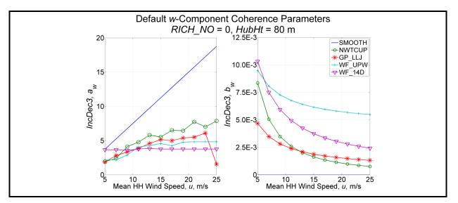
Figure 15. Default *w*-component coherence parameters, *IncDec3*, ( $a_w$  left,  $b_w$  right) as a function of wind speed, using *RICH\_NO* = 0 and *HubHt* = 80 m (IEC does not define *w*-component coherence parameters)
