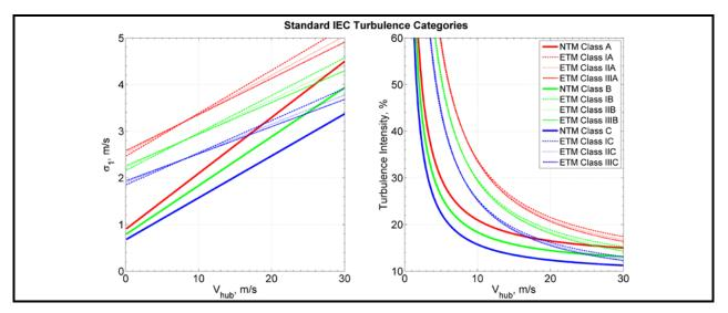
Figure 7. Longitudinal wind-speed standard deviation and TI for IEC turbulence categories as functions of the mean hub-height wind speed,  $V_{hub}$
