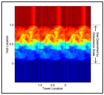
Figure 16. Coherent structure scaling (looking downwind): *CTLy* is the tower location, *CTLz* is the hub (height) location, and *DistScl* determines the size (m) relative to the rotor disk
