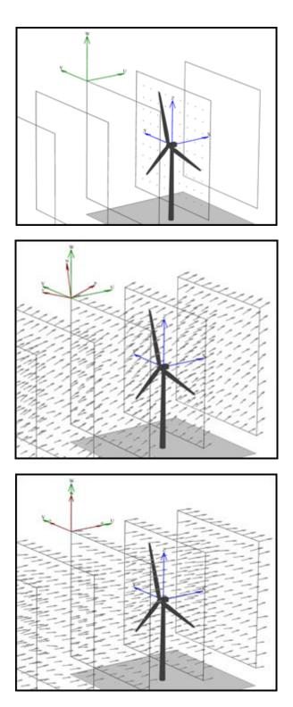
Figure 6. Example of TurbSim grids as implemented in InflowWind: (a) The inertial frame coordinate systems and planes "marching" along positive X, regardless of flow angles, (b) wind field with both flow angles 0°, (c) the same wind field with *VFlowAng* = 8° and *HFlowAng* = 15°
