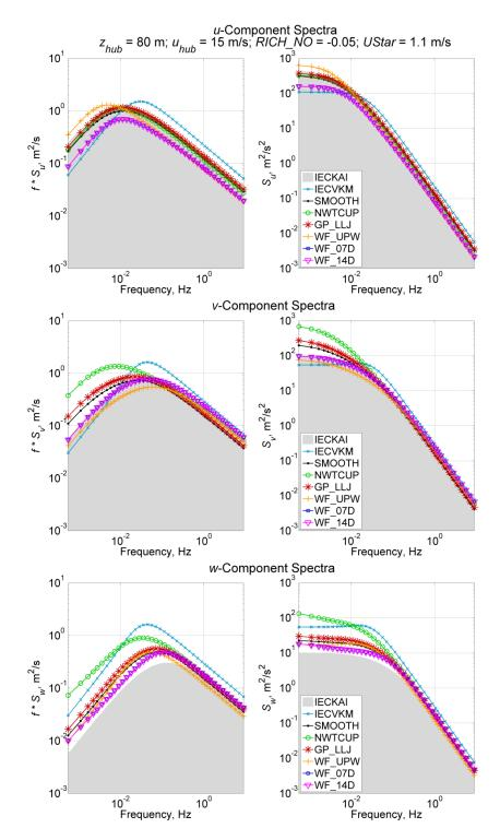
Figure G-6. Unstable velocity spectra using a 15 m/s wind speed at 80 m; the non-IEC models use *RICH\_NO* = -0.05 and *UStar* = 1.1 m/s; the IEC models, which are neutral (*RICH\_NO* = 0), were added for reference; they use NTM category "B" and 61400-1 3<sup>rd</sup> ed. scaling
