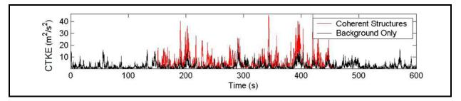
Figure 8. Coherent turbulent kinetic energy (*CTKE*) of an example simulation using KHTEST: the coherent structure placement in the middle of the time series is shown by the red lines
