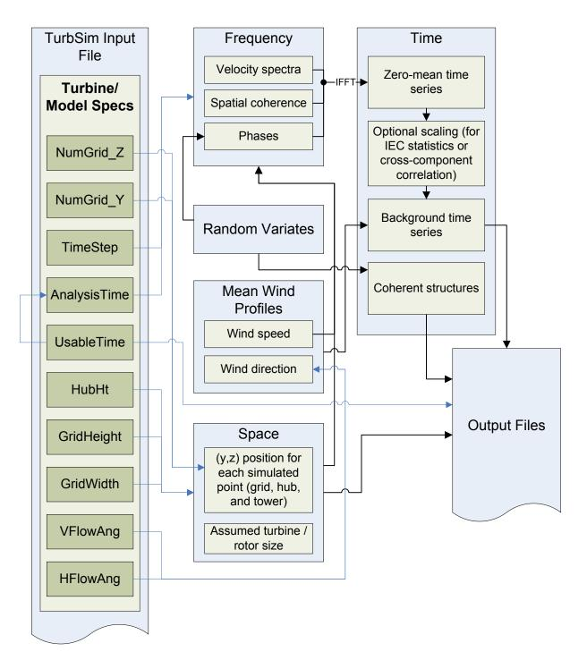
Figure C-3. Parameters in the Turbine/Model Specifications section of the TurbSim input file
