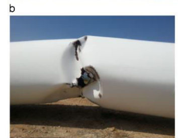
Fig. 10. Tower collapse due to super typhoon Usagi. (a) Tower collapsed towards SW; (b) buckling failure at a tower height of about 9 m.
