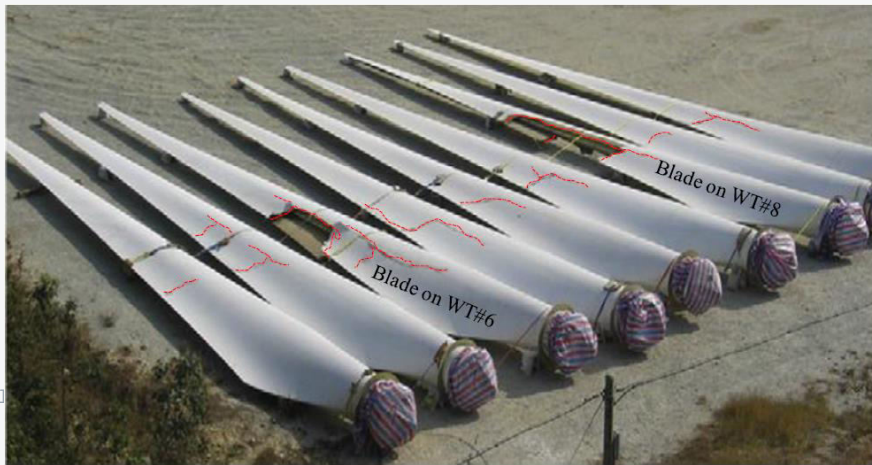
Fig. 8. Rotor blades damaged by super typhoon Dujan in 2003.
