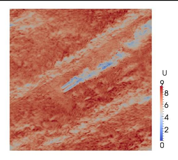
NREL 5MW turbine in unstable high-roughness atmospheric flow with mean speed at 8 m/s @ hub height
