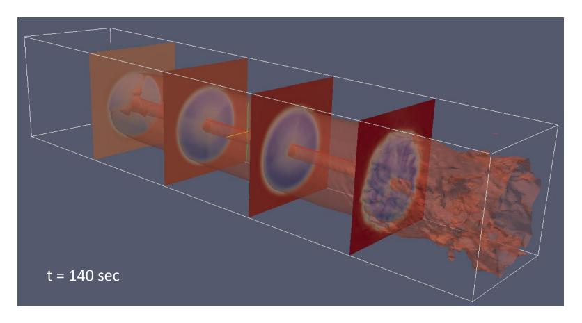
Downstream turbine is being approached with wake structures
