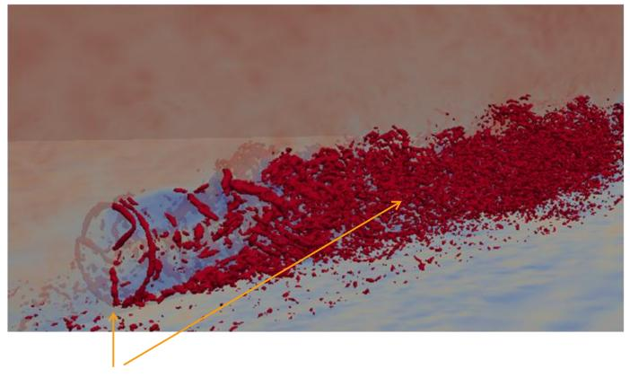
Two NREL 5-MW turbines subjected to neutrally stable low-roughness atmospheric conditions showing the instantaneous streamwise velocity contours with iso-surface of Q invariant fixed at 0.0275 1/s
