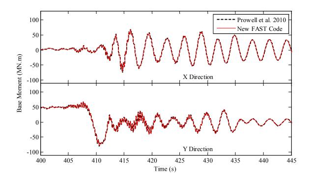
Figure 5. Tower-base moment for emergency shutdown loading condition
