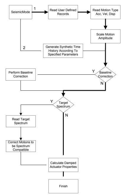
Figure 1. Flowchart for initialization of seismic shaking functionality
