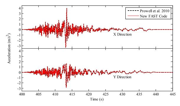
Figure 2. Platform inertial acceleration in idling, operational, and emergency shutdown loading conditions for X and Y directions (EI-Centro earthquake)
