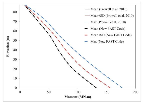
Figure 7. Mean, mean plus standard deviation, and maximum of the SRSS moment for the operational loading condition
