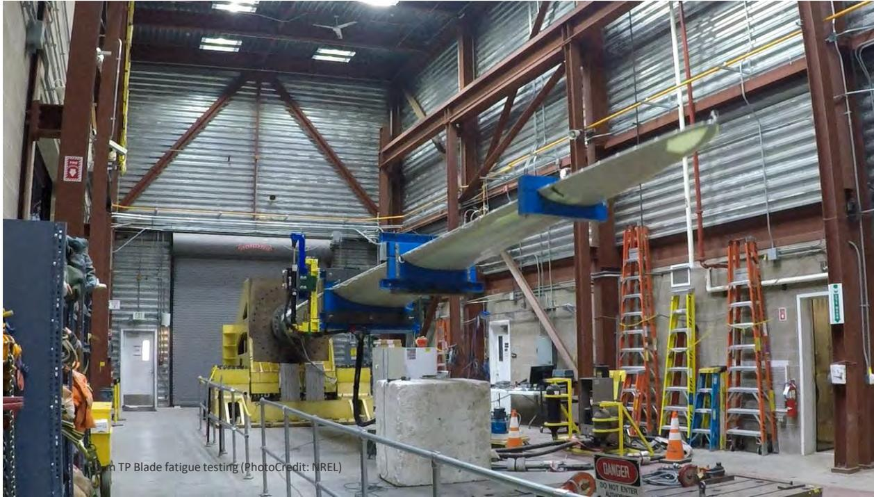
TP Blade fatigue testing (PhotoCredit: NREL)
