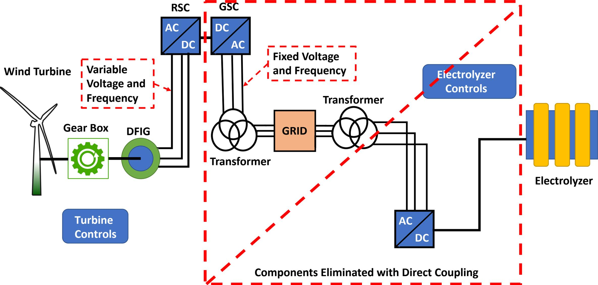
Typical Grid Connected System
