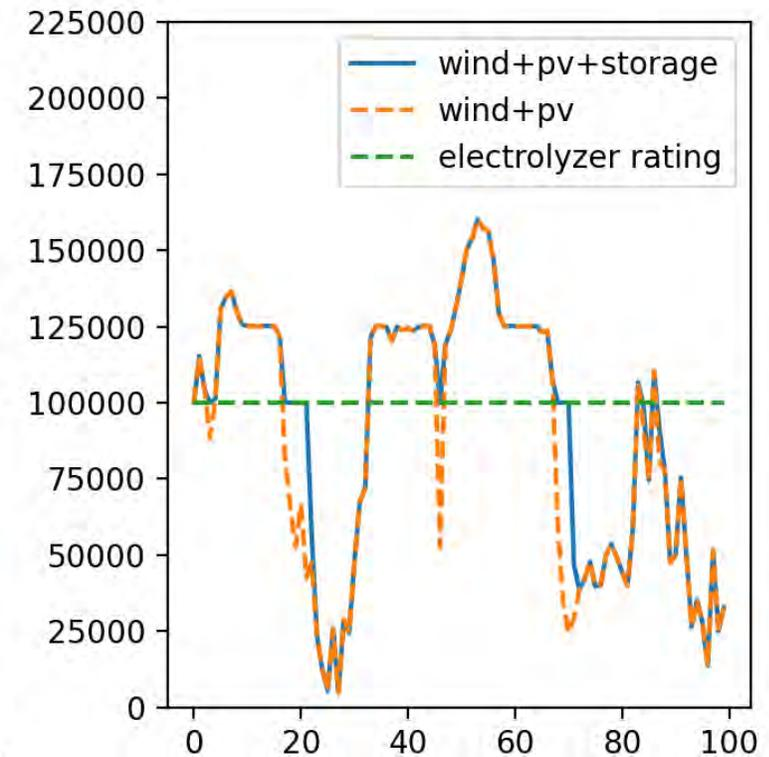
**Battery is not always at max capacity**
