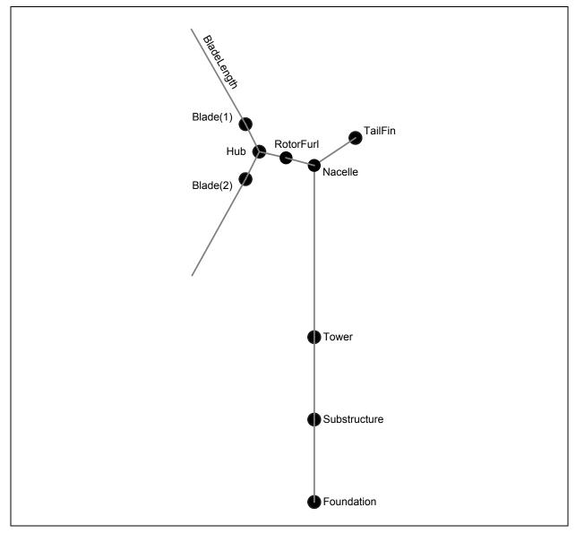
Figure 2. Schematic of AeroConfig data type. Markers give the configuration of the bodies which can influence aerodynamic loads.
