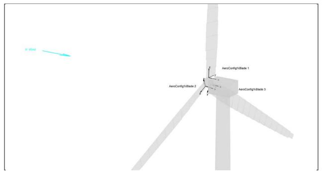
Figure 4. Schematic of AeroConfig%Blade markers for the NREL 5-MW Baseline Onshore Turbine.
