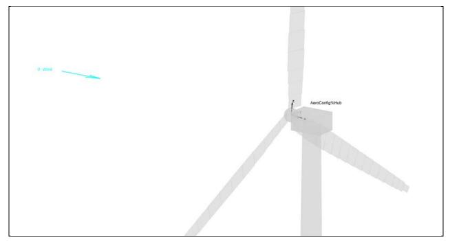
Figure 6. Schematic of AeroConfig%Hub marker for the NREL 5-MW Baseline Onshore Turbine.
