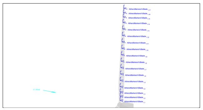
Figure 10. Schematic of AllAeroMarkers%Blade markers for Blade 1 of the NREL 5-MW Baseline Onshore Turbine. This blade has 17 aerodynamic analysis nodes.
