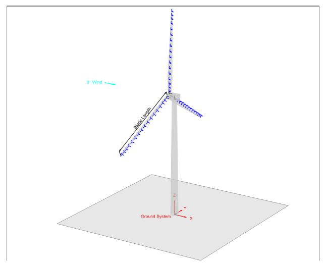
Figure 3. Schematic of AeroConfig (black) and AllAeroMarkers%Blade (blue) markers for the NREL 5-MW Baseline Onshore Turbine. AeroDyn's ground coordinate system is shown in red.
