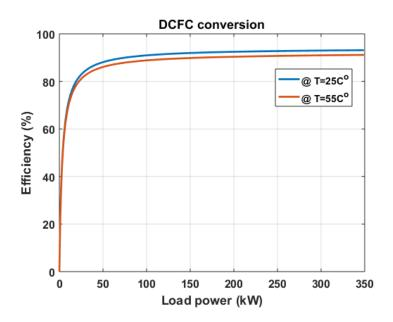
Figure 7. Estimated load-efficiency curves of 550-kVA PV conversion system.
