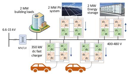
Figure 1. Conventional common AC bus integration.
