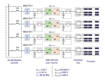
Figure 6. Schematic diagram of conventional ~2-MW PV system.
