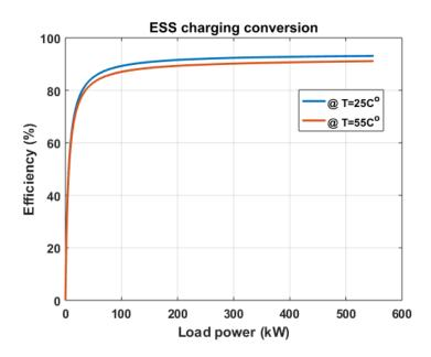
Figure 9. Estimated load-efficiency curves of 540-kVA ESS conversion system during charging.
