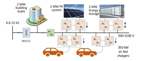
Figure 2. Common DC bus microgrid integration.
