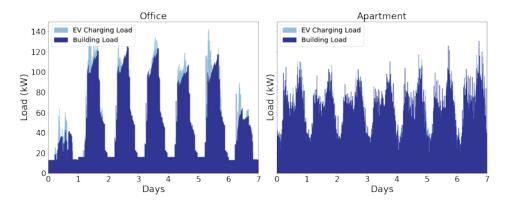
Figure 15. Comparison of office and apartment EV and building load profiles.
