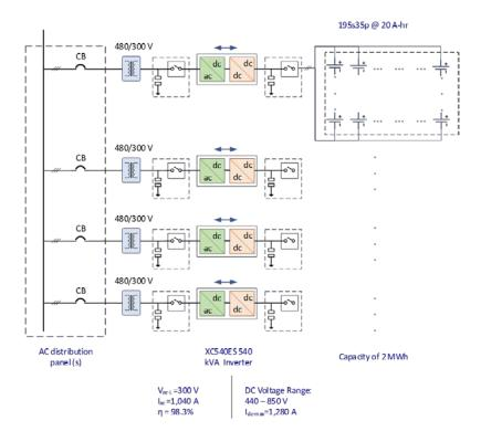
Figure 8. Schematic diagram of conventional ~2-MW ESS system.
