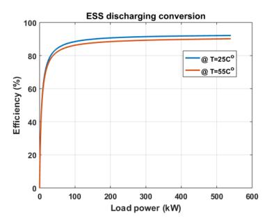
Figure 10. Estimated load-efficiency curves of 540-kVA ESS conversion system during discharging.
