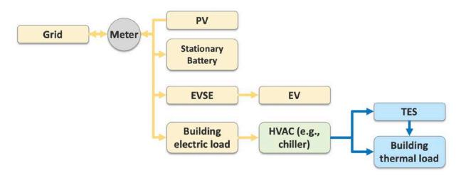
Figure 1. Schematic depicting the default combination of technologies for BTMS analysis.
