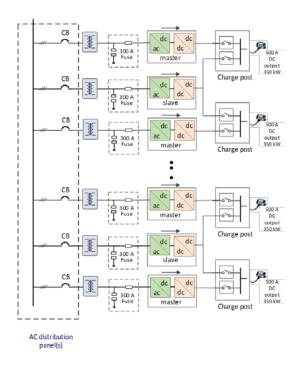
Figure 4. Schematic diagram of conventional ~2-MW DCFCs system.
