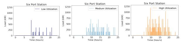
Figure 4. Schematic depicting how station utilization affects the load profile for a six-port station.
