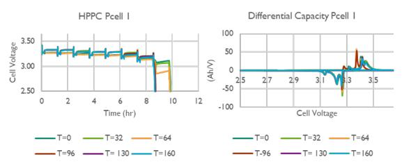
Figure 4. Power cell 1 state-of-health testing of LFP/graphite cells.
