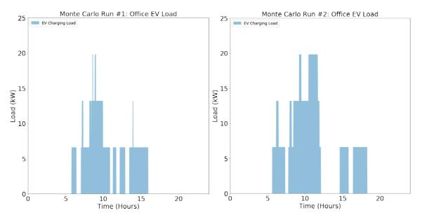
Figure 8. Schematic depicting two Monte Carlo simulations to generate EV profiles for an office station.
