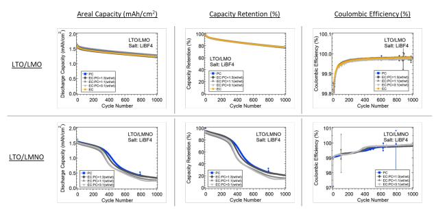
Figure 4. Cycle performance of LTO/LMO (top row) and LTO/LMNO (bottom row) cells with LiBF<sub>4</sub> salt in a series of EC-PC solvent mixtures. Cells were cycled at C/10 for 2 formation cycles and at 1C for aging cycles. LTO/LMO cells were cycled between 1.5 and 3.0 V, and LTO/LMNO cells were cycled between 1.5 and 3.5 V.
