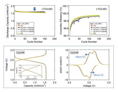
Figure 5. Cycle performance of LTO/LMO cells with LiPF<sub>6</sub> salt in a series of EC-PC solvent mixtures (top row). Cells were cycled at C/10 for 2 formation cycles and at 1C for aging cycles between 1.5 and 3.0 V. Voltage profiles and dQ/dV plots of the 100<sup>th</sup> cycle in each system are shown in the bottom row.
