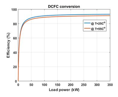
Figure 5. Estimated load-efficiency curves of 350-kW DCFC conversion system.
