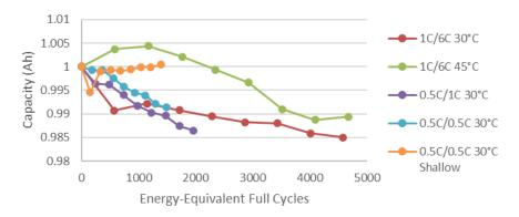
Figure 2. LTO/NMC cycle life capacity loss for a variety of rates and temperatures.
