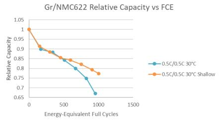
Figure 1. Graphite/NMC622 0.5C/05C full-depth and shallow cycle life capacity retention at 30°C.
