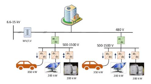
Figure 3. Modular-based multiple DC bus microgrid integration.
