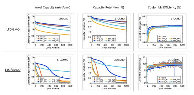
Figure 3. Cycle performance of LTO/LMO (top row) and LTO/LMNO (bottom row) cells with LiPF<sub>6</sub> and LiBF<sub>4</sub> in PC and FEC electrolytes. Gen2 electrolyte is shown as comparison. Cells were cycled at C/10 for 2 formation cycles and at 1C for 1000 aging cycles. LTO/LMO cells were cycled between 1.5 and 3.0 V, and LTO/LMNO cells were cycled between 1.5 and 3.5 V.
