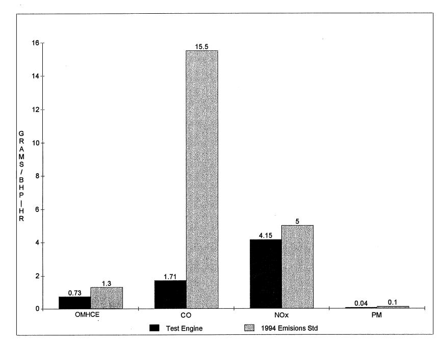
Figure 6. Ethanol 6V-92TA Engine Certification Data
