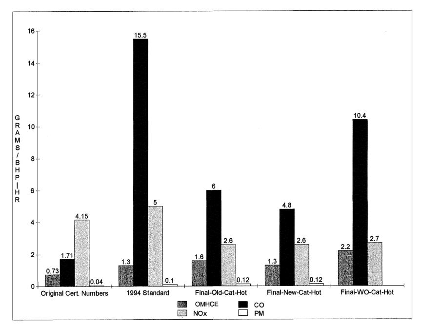
Figure 7. Final Emissions Data (Hot Engine)
