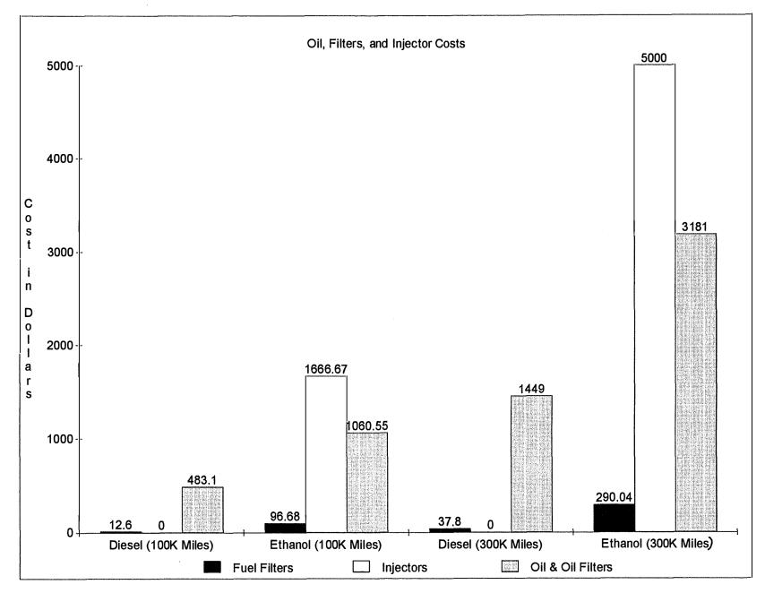
Figure 11(b). Oil, Filter, and Injector Costs
