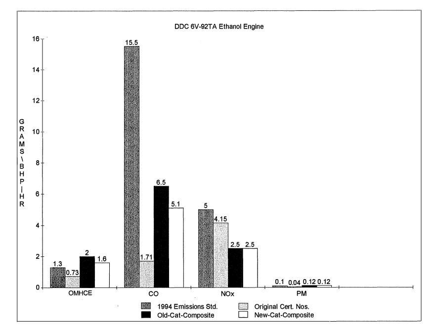
Figure 8. Final Emissions Data (Composite)
