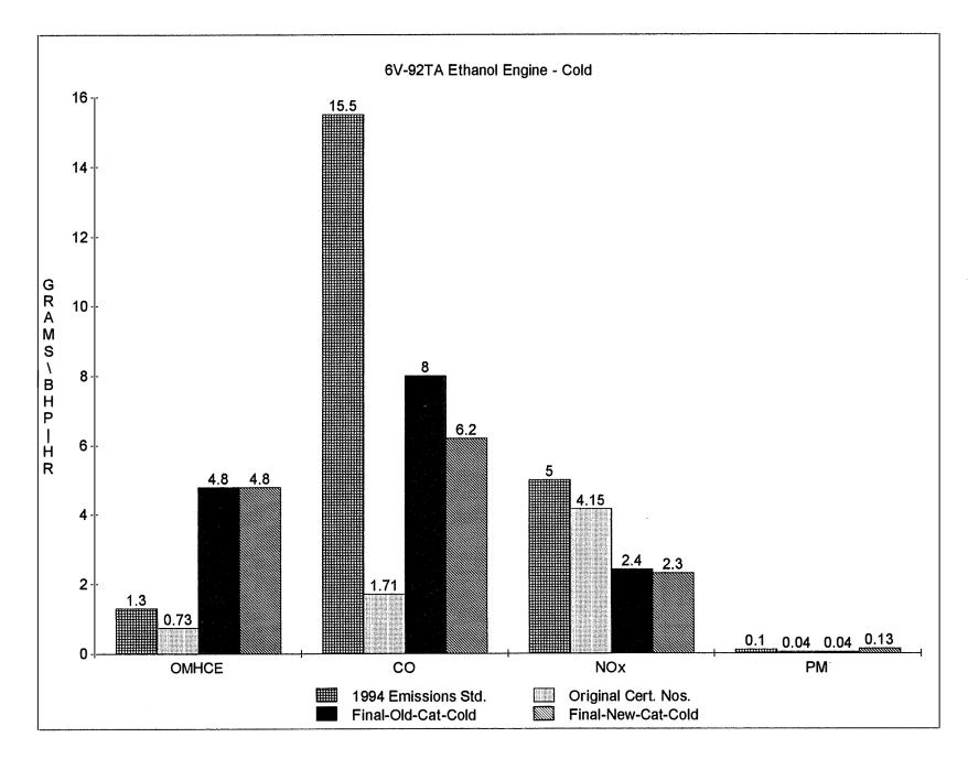
Figure 9. Final Emissions Data (Cold Engine)
