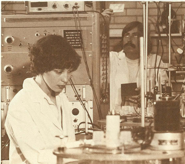
Researchers are making electrochemical measurements to determine corrosion rates of materials used in solar collectors.
