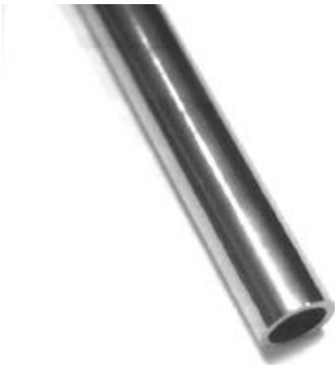
Fig. 6. A 6-mm-diameter silicon tube with approximately 0.7-mm wall thickness grown from a capillary die.
