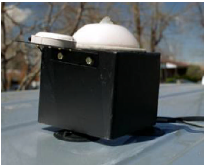
Figure 8: Close-up View of the Antennas for Two-Way Communication (large dome) and for GPS (small disc)
