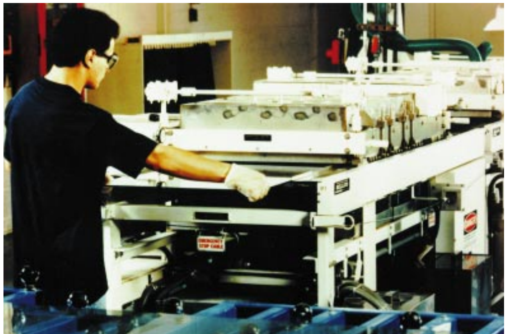
Glass-washing step in SCI's module manufacturing line.
