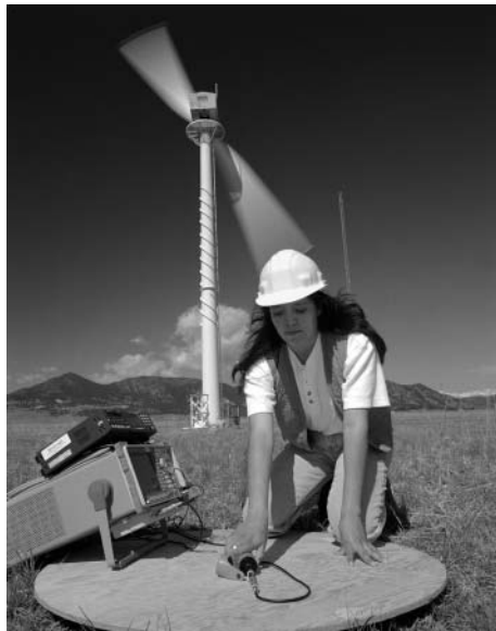
Certification test engineer measures noise emissions from a wind turbine at the National Wind Technology Center.
